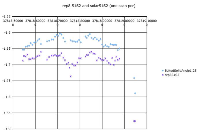
Figure 5: A comparison of  $Z_{dr}$  bias monitoring via test pulse injection (purple markers) and sun scans (blue markers). The horizontal axis is in Unix days and the vertical axis is in dB. Data was gathered on 17 July 2007.
