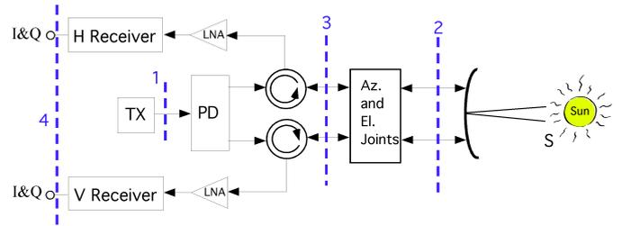
Figure 1: A block diagram of a radar system for the EC method.
