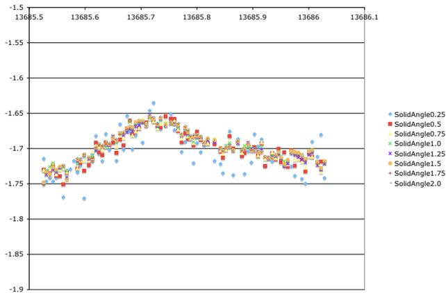
Figure 3:  $S_1S_2$  sun scan measurements over an entire day for various solid angles of integration.
