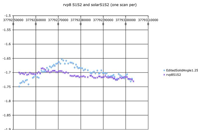
Figure 6: A comparison of  $Z_{dr}$  bias monitoring via test pulse injection (purple markers) and sun scans (blue markers). The horizontal axis is in Unix days and the vertical axis is in dB. Data was gathered on 21 June 2007
