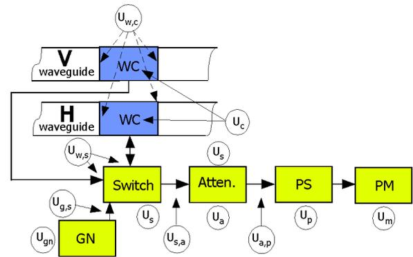
Figure 2: A block diagram of a differential waveguide power measurement. "WC" is waveguide coupler, "Atten." is an attenuator, "PS" is a power sensor, "PM" is a power meter and "GN" is a generator. The circles represent the various uncertainties. The double subscripted uncertainties are various impedance mismatches between the devices. A list of the uncertainties with definitions is given in Table 1
