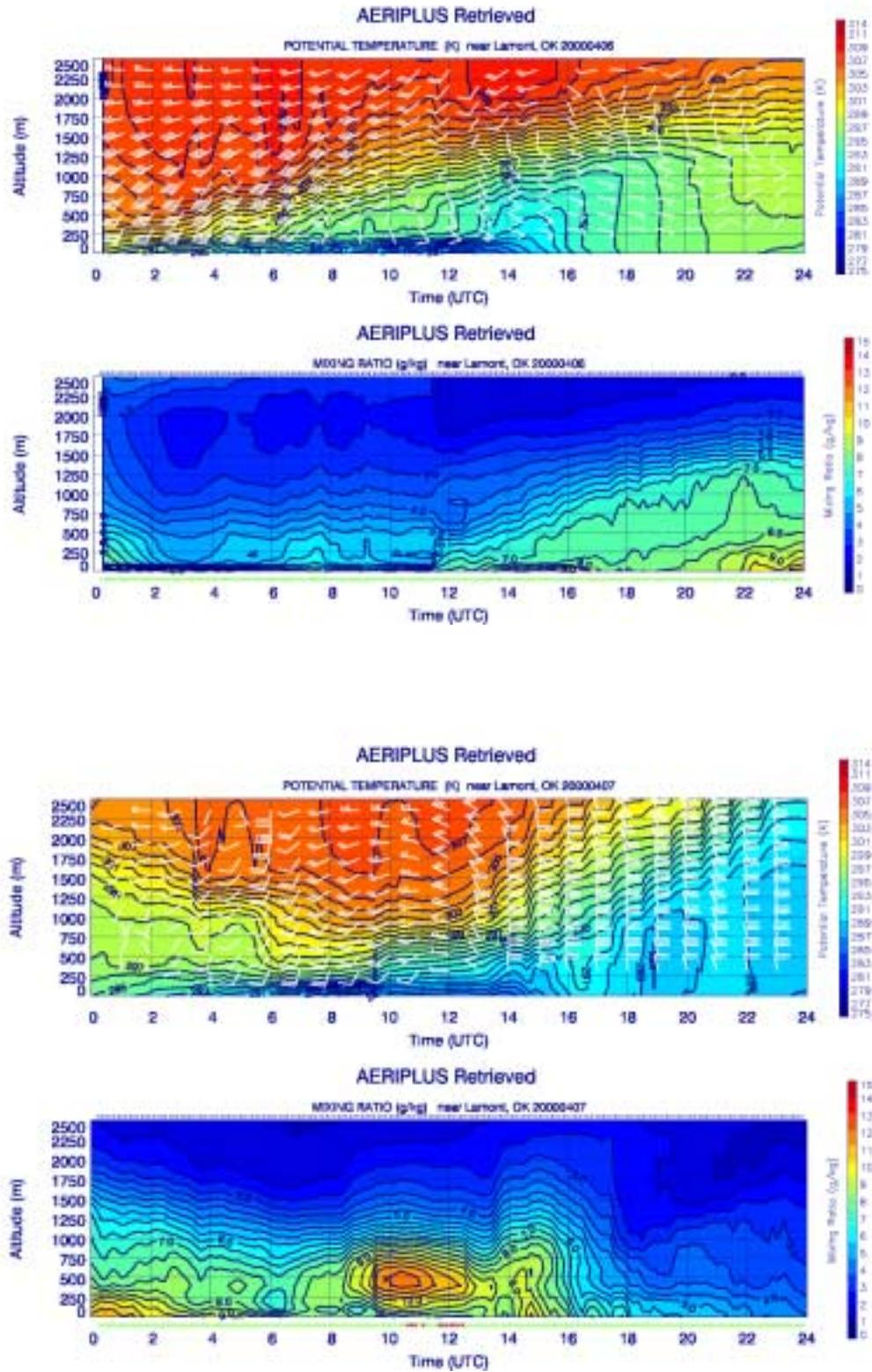
**Figure 8:** Potential temperature and water vapor mixing ratio measured by AERI at the ARM central facility showing frontal passages on 6 and 7 April 2000. The overlaid winds are from the Lamont wind profiler. (modified 1 Feb 2001)
