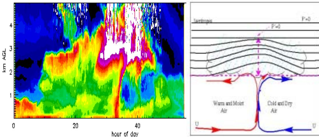
**Figure 11:** Schematic diagram showing a symmetric convergence line in a stratified atmosphere and relative humidity profile derived from the Raman lidar measured water vapor mixing ratio data on 28 September 1997 by the ARM lidar (CARL). The location of the clouds, the narrow convergence zone and lifting associated are all visualized in detail. Figure and caption provided by B. Demoz, U Maryland at Baltimore County.
