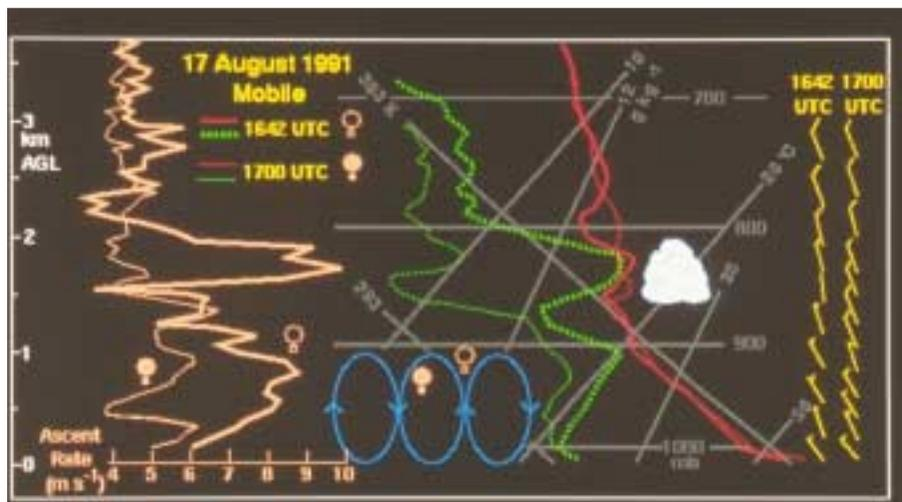
**Figure 4:** Ascent rate, water vapor mixing ratio, temperature and winds from two rawinsondes launched through a convective boundary layer in Florida. Although the soundings were taken only 18 minutes apart there are significant differences, particular in the mixing ratios. The reason for this difference is that one sonde ascended through the updraft of a convective roll, while the drier sounding was taken within a roll downdraft. Weckwerth et al. (1996).
