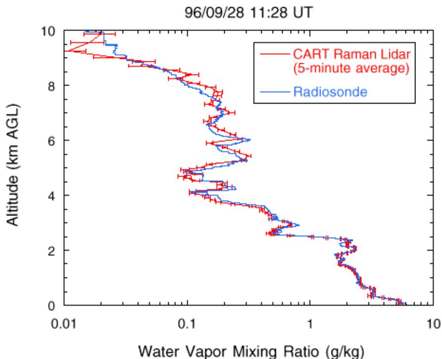
Figure 9: Comparison between the ARM CART Raman lidar and a Vaisala radiosonde launched from the CART site on 1128 UTC on 28 September 1996.
