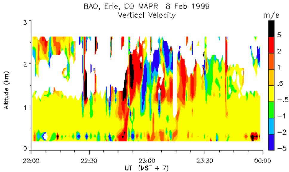
**Figure 12:** Vertical air motion from MAPR (Multiple Antenna Profiler) through a cold front. MAPR is also capable of measuring the horizontal winds at high-resolution (30s to several mins) and RASS measurements of virtual temperature. Courtesy of W. Brown, NCAR.
