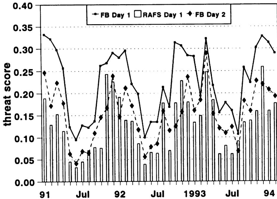
**Figure 1:** Monthly threat scores for quantitative precipitation forecasts at the 1'' or greater threshold for the period from January 1991 through January 1994. Threat scores are plotted for the NGM/RAFS models for the 0 to 24-h period and for forecaster based (FB) predictions at the 0 to 24-h and 24 to 48-h. Adapted from Uccellini et al (1994).
