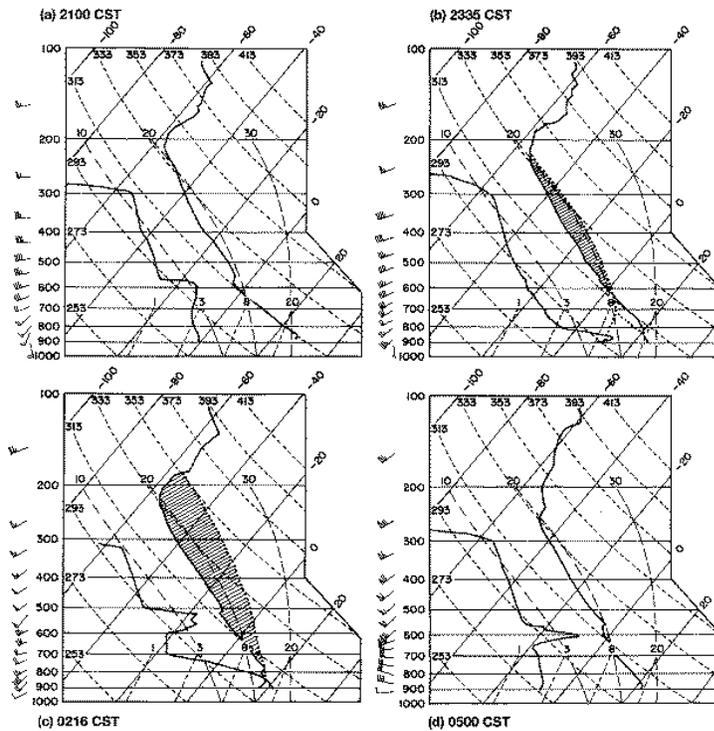
**Figure 6:** Serial radiosonde ascents from the event shown in Fig. 5. The increase in integrated water vapor corresponded to a rapid destabilization as the CAPE increased nearly 3000 J kg<sup>-1</sup> in less than 3 hrs between 2335 and 0216 CST in a nocturnal environment (Parsons et al. 2000).
