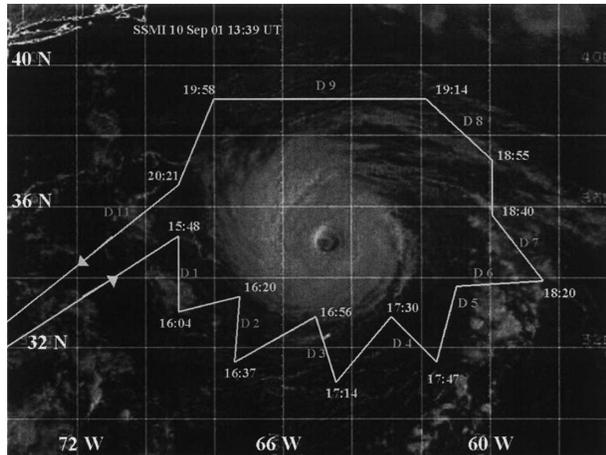
FIG. 7. The flight track of the NASA DC-8 around Hurricane Erin on 10 Sep 2001. Aircraft turn times are noted as are the locations of the eleven dropsonde releases depicted with D# notation. Image courtesy of R. Ferrare/NASA Langley Research Center.
