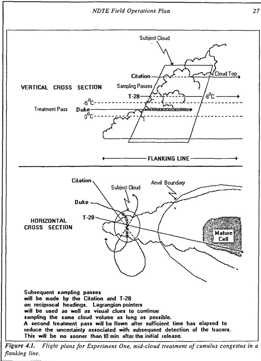
**Figure 3.** Schematic for Experiment 1 as it appeared in the Field Operations Plan.
