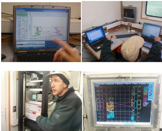
*Onboard the MISS (Top left to bottom right: Live streaming radiosonde data – Ceilometer data left screen and radiosonde data right screen – Lou showing us the radiosonde amplification and GPS hardware – Temperature, dew point, relative humidity, wind speed and direction readouts.)*
