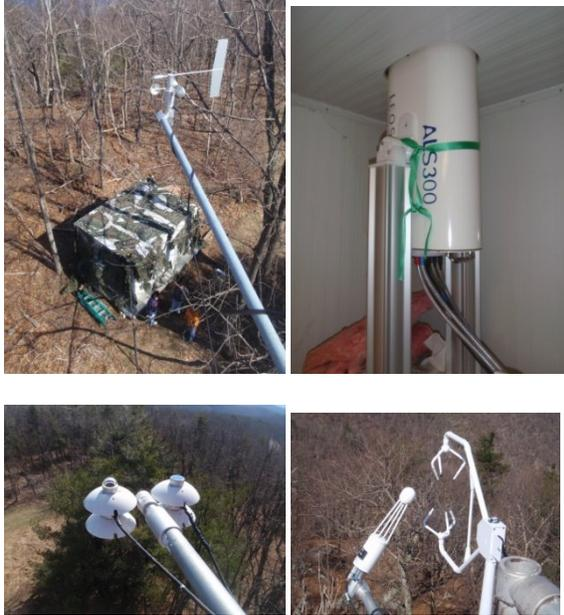
*Pinnacles tower instruments (Top left to bottom right: 3-cup anemometer with computer shed in background – LIDAR – Net radiometer – On the left, open path gas analyzer; on the right, sonic anemometer.)*
