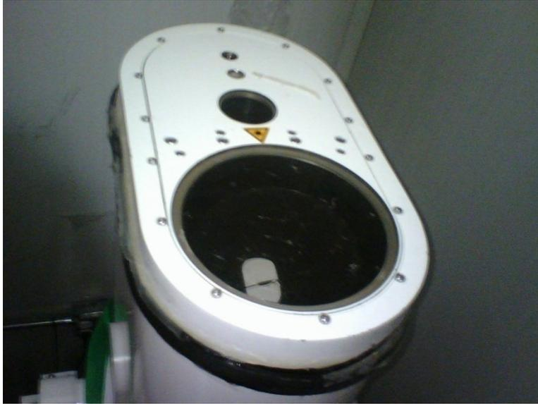
UVA LIDAR. The small hole is the transmitter and the large hole is the receiver.
