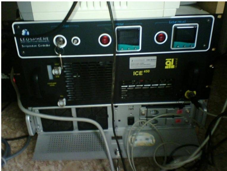
The top box maintains a constant temperature inside the LIDAR, the middle box controls the laser firing, and the bottom is the CPU for data collection.
