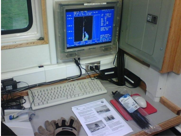
MISS control room. The screen is displaying real-time radar data
