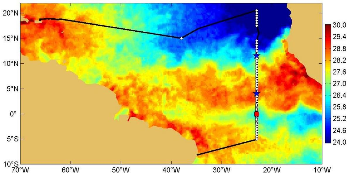
Fig. 2: cruise track of the R/V Ronald H. Brown during leg 1 (black), with CTD stations (white bullets), PNE deployment sites (blue stars), and the PIRATA backbone servicing site (red square). Background shading is SST (°C) on 13 June 2006, from merged TMI/AMSRE microwave satellite observations (Remote Sensing Systems).
