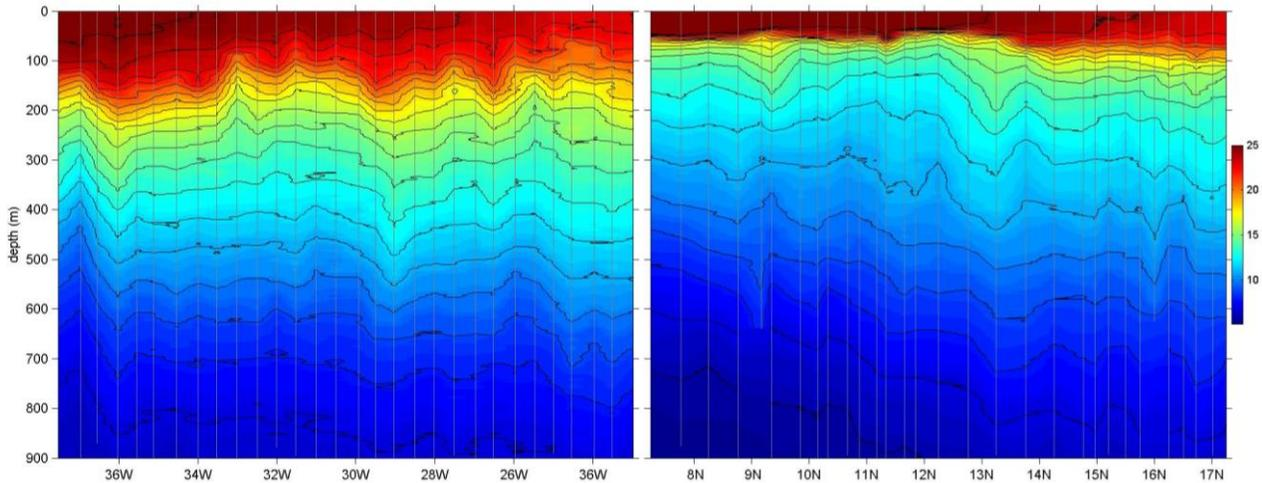
Fig. 8: temperature sections ( $^{\circ}\text{C}$ ) from XBT deployments. Left: almost zonal section from  $37^{\circ}32'\text{W}$  to  $22^{\circ}59'\text{W}$ ,  $10\text{--}20^{\circ}\text{N}$ . Right: meridional section from  $17^{\circ}15'\text{N}$  to  $7^{\circ}15'\text{N}$ ,  $\sim 23^{\circ}\text{W}$ .
