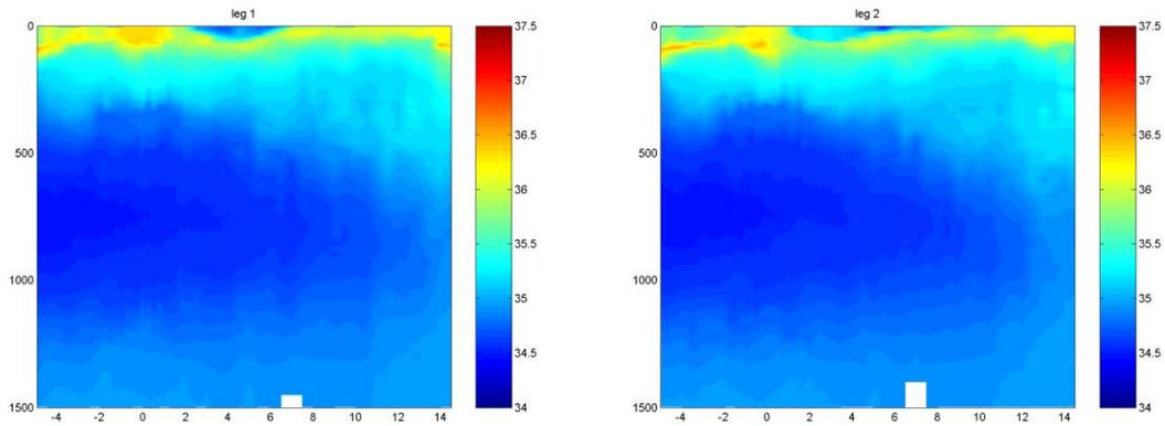
Fig. 5: sections of salinity along 23°W collected during leg 1 (left) and leg 2 (right).
