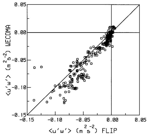
FIG. 18. A comparison of measurements of the longitudinal component  $\langle u'w' \rangle$  of the momentum flux taken from the R/V *Wecoma* and R/P *FLIP*. The data represent 30-min averages computed when the R/V *Wecoma* was within 50 km of the R/P *FLIP*.
