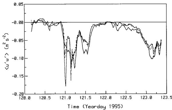
FIG. 17. A time series of the longitudinal component  $\langle u'w' \rangle$  of the momentum flux measured aboard the R/P *FLIP* and R/V *Wecoma* during a 3-day period in May 1995. The dotted and dashed lines represent measurements taken at 8.7 and 13.8 m aboard the R/P *FLIP*, respectively. The solid line represents the R/V *Wecoma* data.
