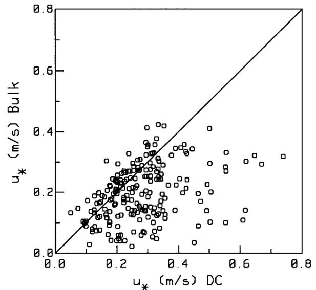
FIG. 12. A comparison of the uncorrected friction velocity estimates from the R/V *Iselin* computed from Eq. (27) vs our bulk aerodynamic estimates. The fluxes represent 30-min averages computed from three 10-min estimates.
