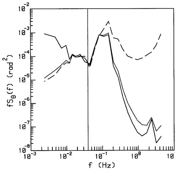
FIG. 1. The variance spectra of our angular estimates of  $\theta$ . The broken line is computed from  $-x/g$ , the solid line is computed from a time series of the integrated rate sensor, and the dotted line is computed using complementary filtering. The vertical line in the figure shows the location of our cutoff frequency  $f_m/5$ .
