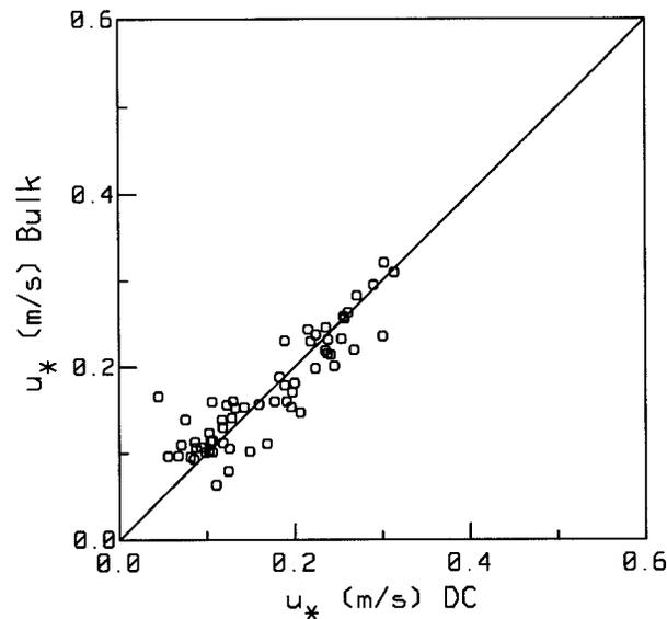
FIG. 11. A comparison of the corrected friction velocity estimates from the R/P *LADAS* computed from Eq. (27) vs our bulk aerodynamic estimates. The fluxes represent 30-min averages computed from three 10-min estimates.
