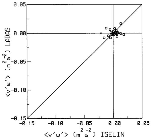
FIG. 15. A comparison of measurements of the lateral component  $\langle v'w' \rangle$  of the momentum flux taken from the R/V *Iselin* and R/P *LADAS*. The data represent 30-min averages where there is at least 20 min of overlap between the estimates.
