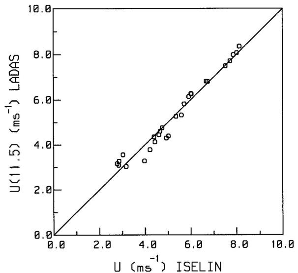
FIG. 16. A comparison of our relative wind speed measurements taken from the R/V *Iselin* and R/P *LADAS*. The R/P *LADAS* measurements have been adjusted to the height of the R/V *Iselin* measurements using the friction velocity and stability corrections computed using the bulk aerodynamic method of Fairall et al. (1996).
