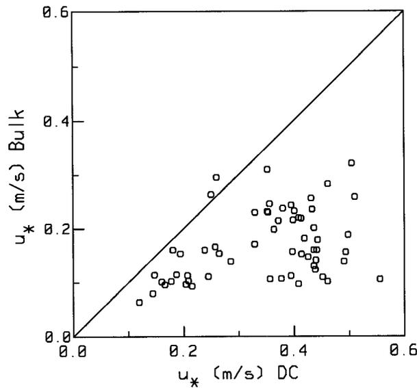
FIG. 10. A comparison of the uncorrected friction velocity estimates from the R/P *LADAS* computed from Eq. (27) vs our bulk aerodynamic estimates. The fluxes represent 30-min averages computed from three 10-min estimates.
