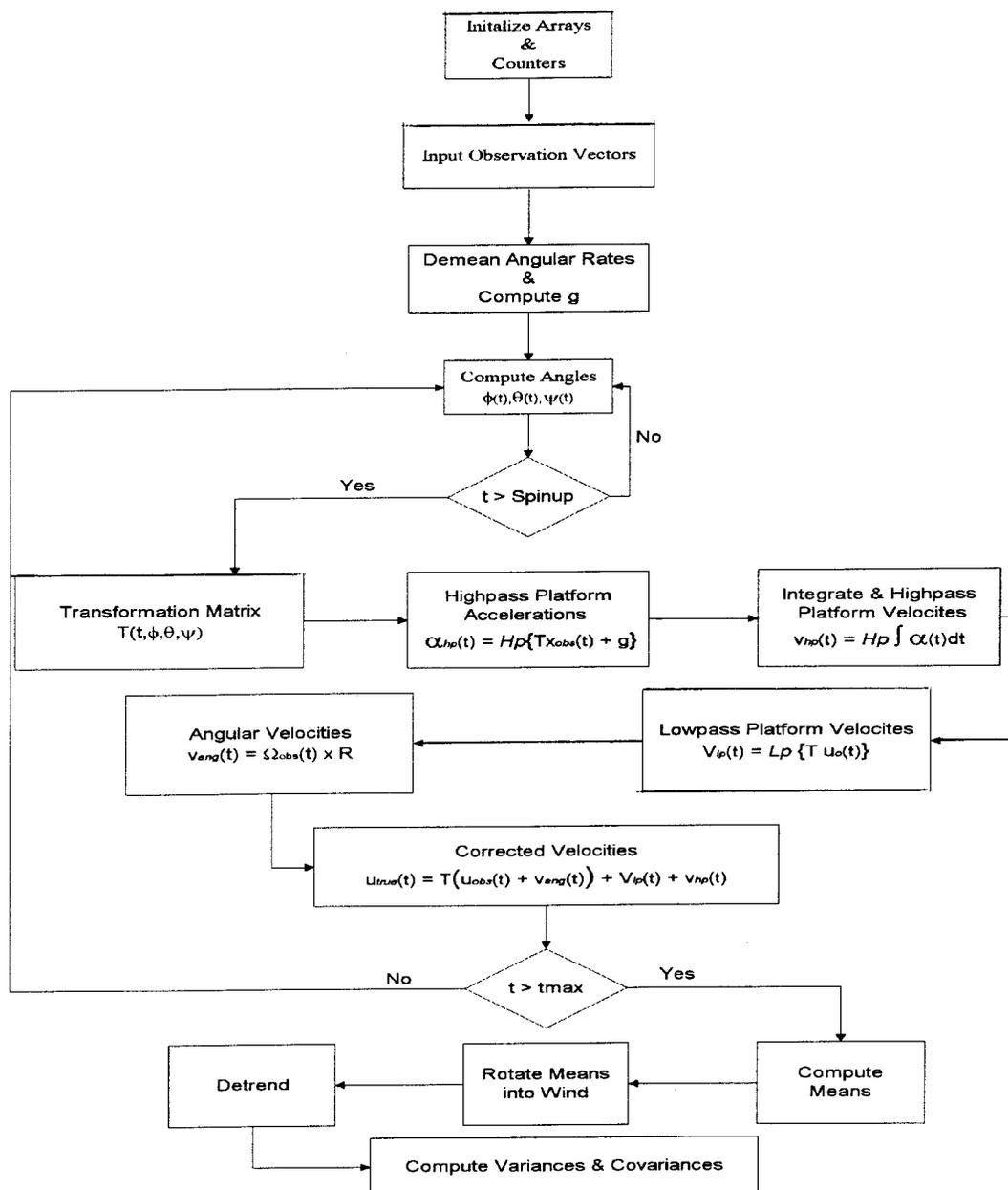
FIG. 2. A flowchart of the method used to postprocess the data. Spinup represents the time given to the complementary filters to provide the proper angles, while  $t_{max}$  represents the record length.
