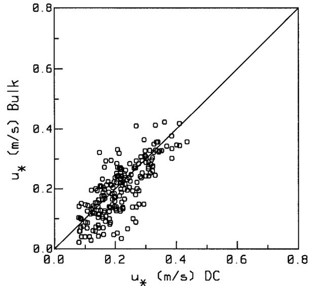
FIG. 13. A comparison of the corrected friction velocity estimates from the R/V *Iselin* computed from Eq. (27) vs our bulk aerodynamic estimates. The fluxes represent 30-min averages computed from three 10-min estimates.
