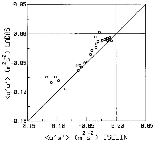
FIG. 14. A comparison of measurements of the longitudinal component  $\langle u'w' \rangle$  of the momentum flux taken from the R/V *Iselin* and R/P *LADAS*. The data represent 30-min averages where there is at least 20 min of overlap between the estimates.
