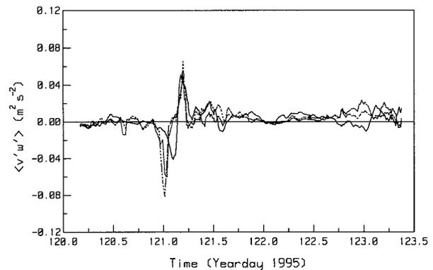
FIG. 22. A time series of the lateral component  $\langle v'w' \rangle$  of the momentum flux measured aboard the R/P *FLIP* and R/V *Wecoma* during a 3-day period in May 1995. The dotted and dashed lines represent measurements taken at 8.7 and 13.8 m aboard the R/P *FLIP*, respectively. The solid line represents the R/V *Wecoma* data.
