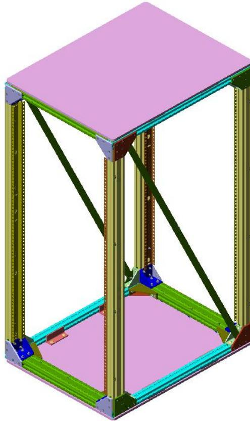
**Figure 5.3. Standard GV Equipment Rack**
