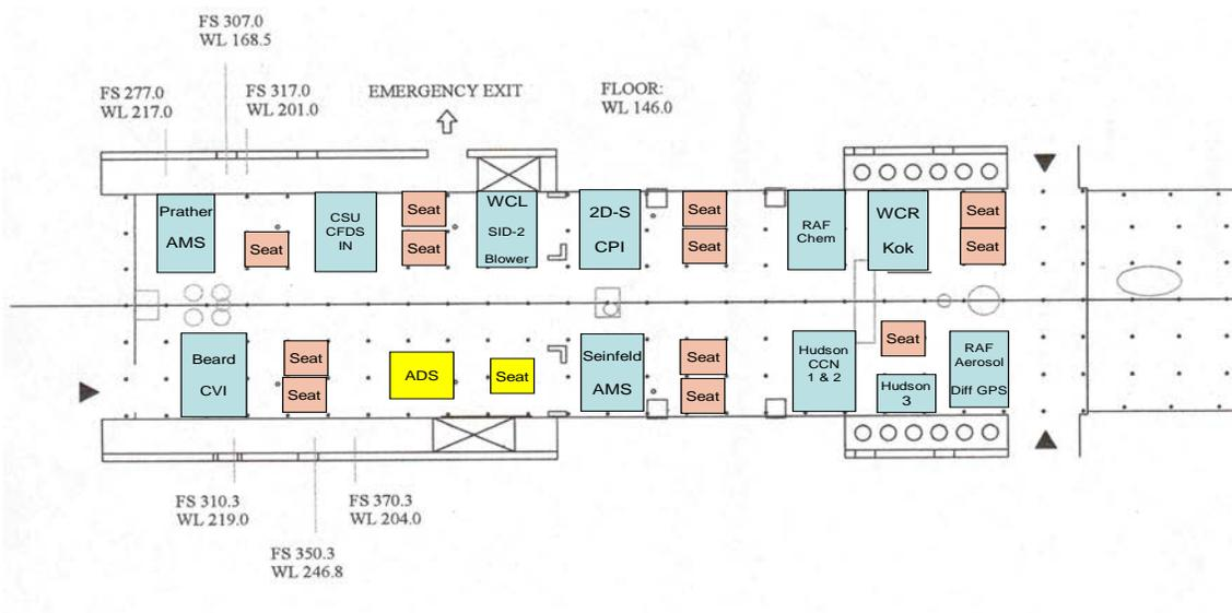
Figure 5.1 Typical Research Cabin Configuration
