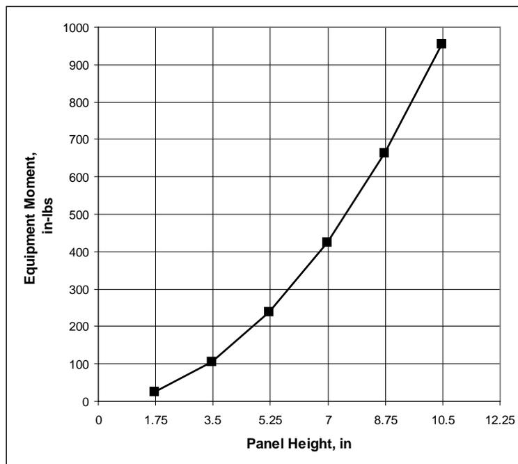
**Figure 5.5. Allowable face-mounted equipment moment chart.**
