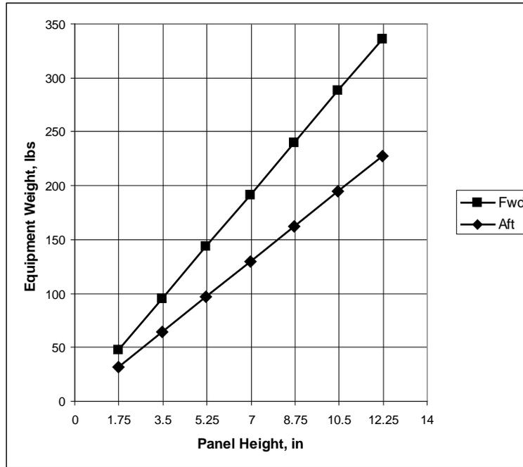
**Figure 5.4. Allowable equipment weight for mounting to face chart.**
