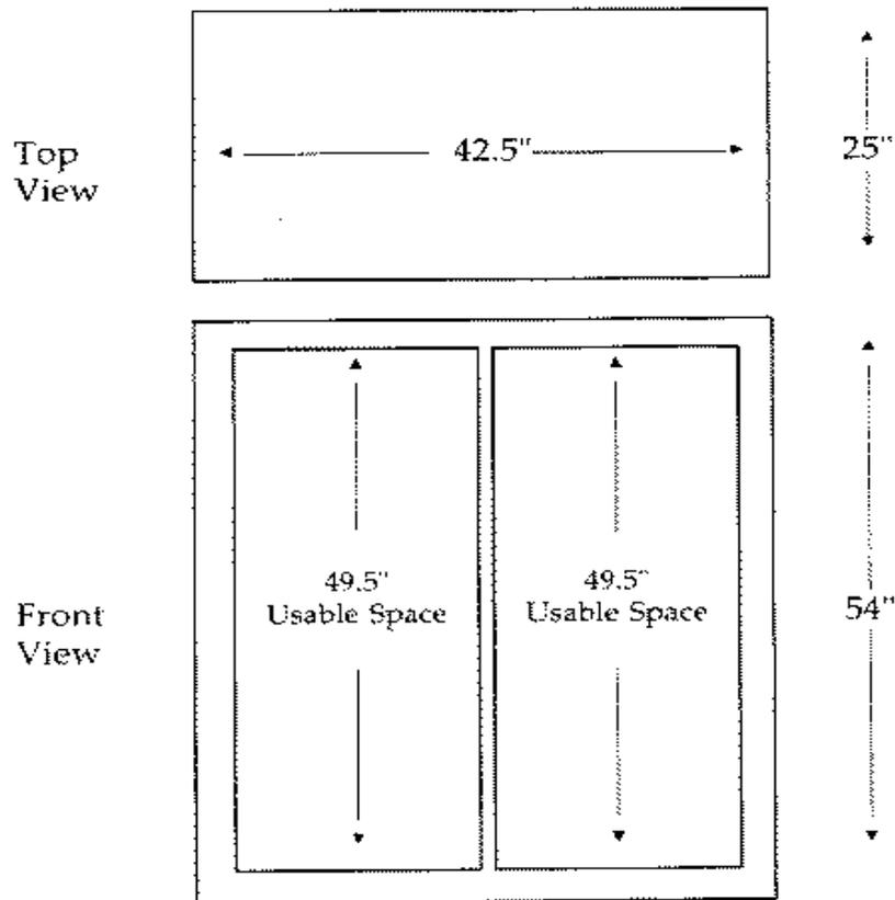
Figure 5.2. Standard C-130 Equipment Rack; each bay is 19" wide.
