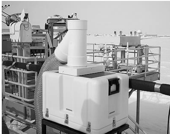
Fig. 6. The prototype Ground-based GVR at the DOE North Slope of Alaska "Great White" site near Barrow, Alaska. A tilted 1 mil. Mylar film radome window is kept clear from rain or snow with a 500 CFM blower and hood.
