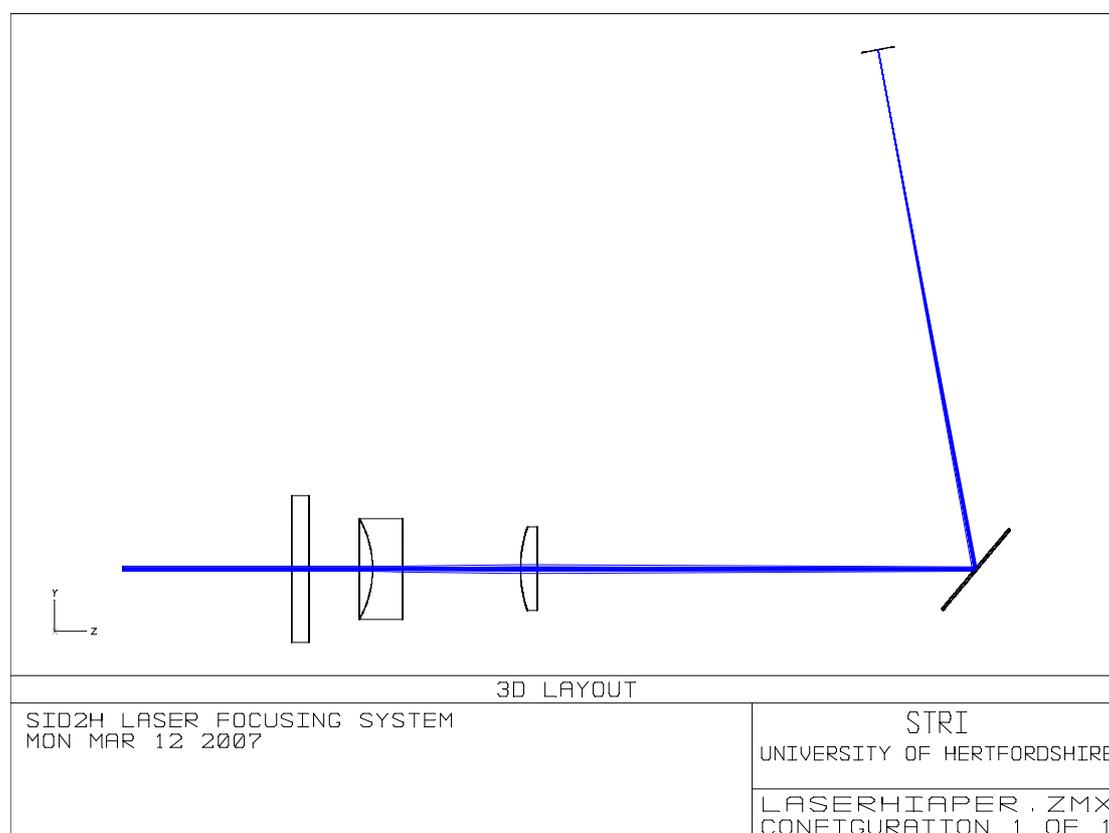
Figure 1. Beam shaping optics.
