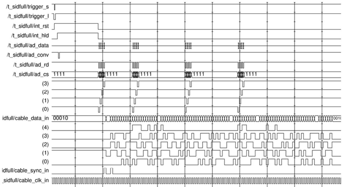
Figure 6. PFGA timing diagram for data capture and transmission.
