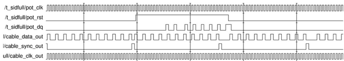
Figure 7. Timing diagram for writing to the digital potentiometers.
