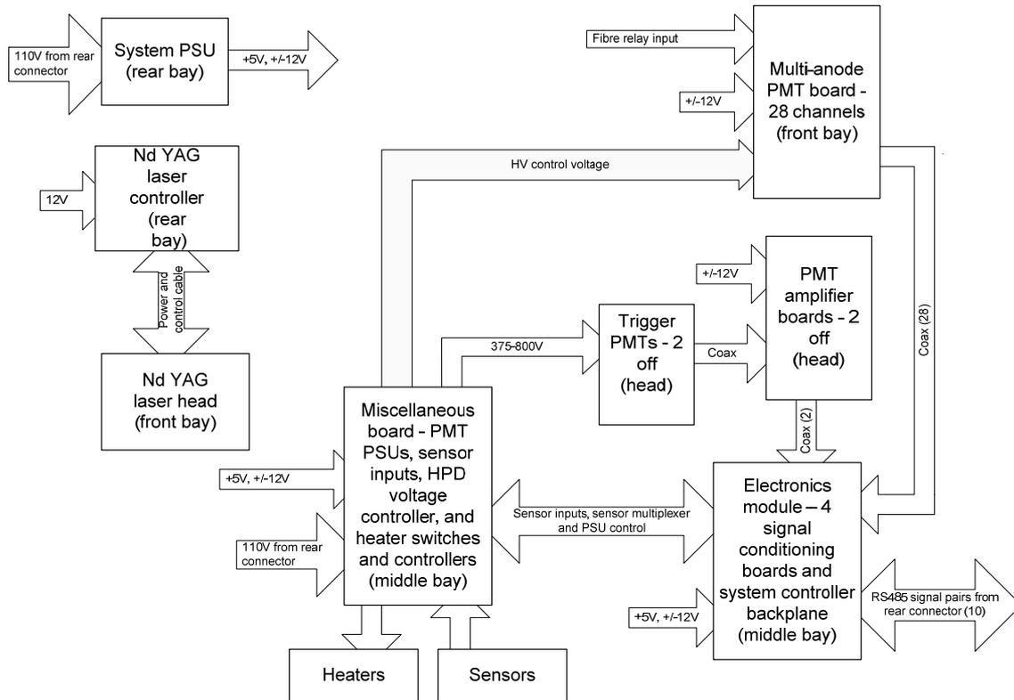
Figure 4. Electrical connectivity.
