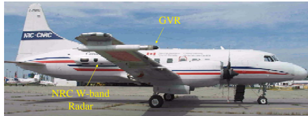
Figure 1. The NRC Convair-580 aircraft with the NAWX radar system and G-band water Vapor Radiometer (GVR).
