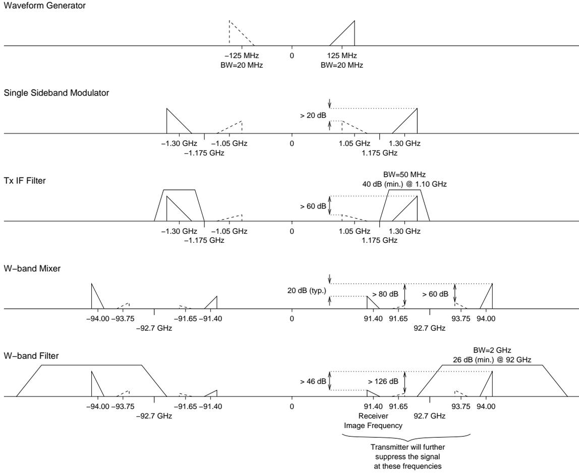
Figure 8: Two stage heterodyne frequency up-conversion.
