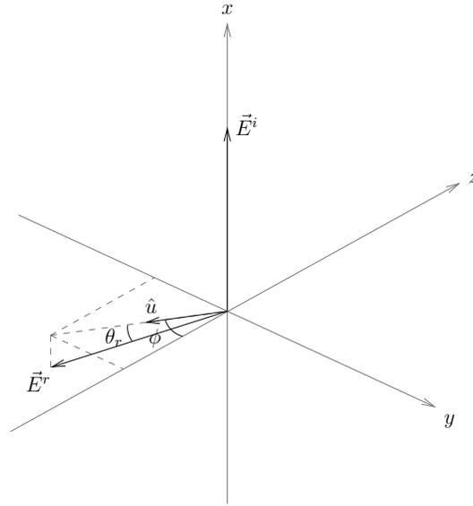
Figure 5: Incident and reflected electric field vectors for a reflector plate that is rotated by an angle  $\phi$ . The incident electric field is orientated along the x axis, and the reflected electric field is rotated by an angle  $\phi$  from the xz plane, and by an angle  $\theta$  from the yz plane.
