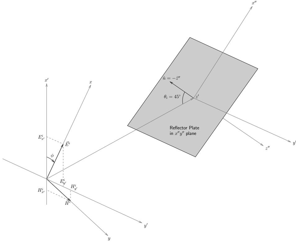
Figure 4: Incident electric field on reflector plate.
