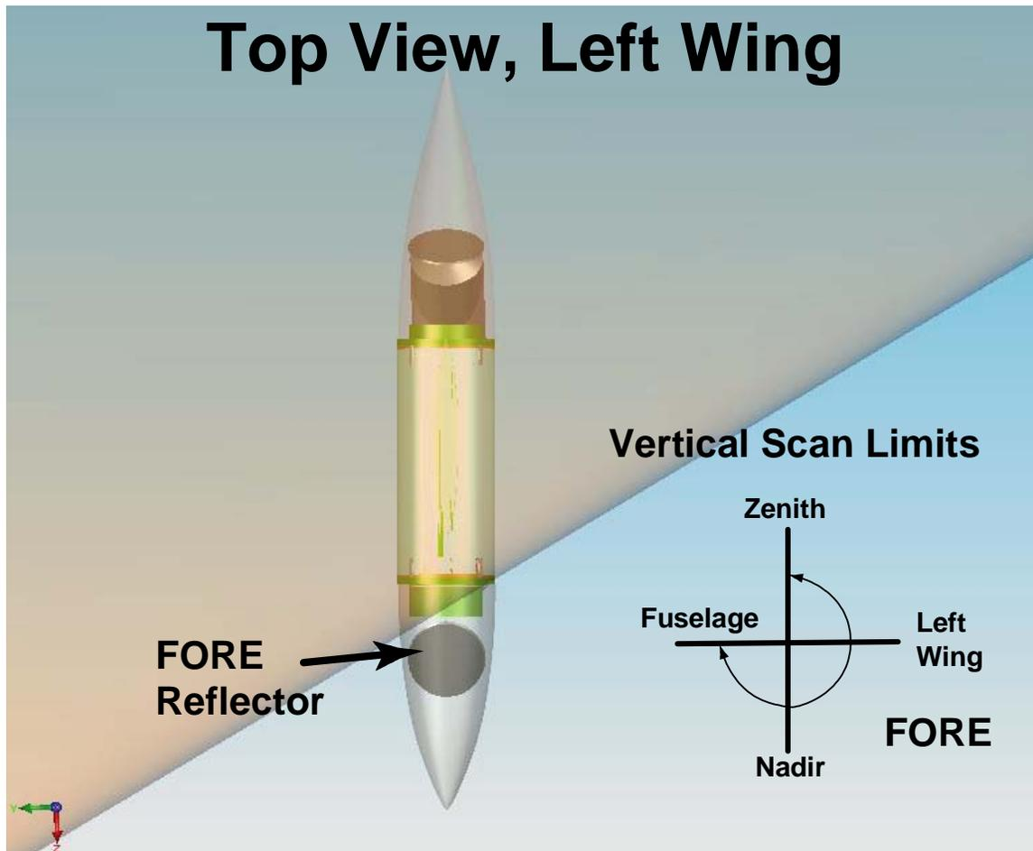
Figure 1: The radar will be able to scan from zenith to through nadir, and towards to the fuselage of the aircraft.
