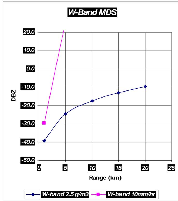
Figure 12: Minimum detectable signal versus range.
