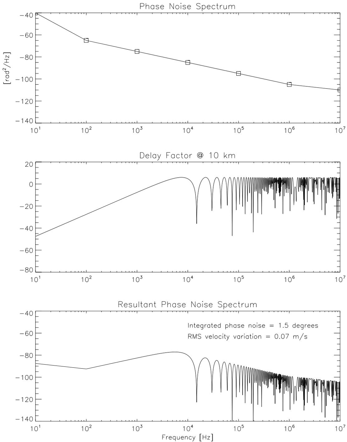
Figure 10: Specification of W-band local oscillator phase noise spectrum and resultant RMS velocity uncertainty due to local oscillator instability for features at 10 km.
