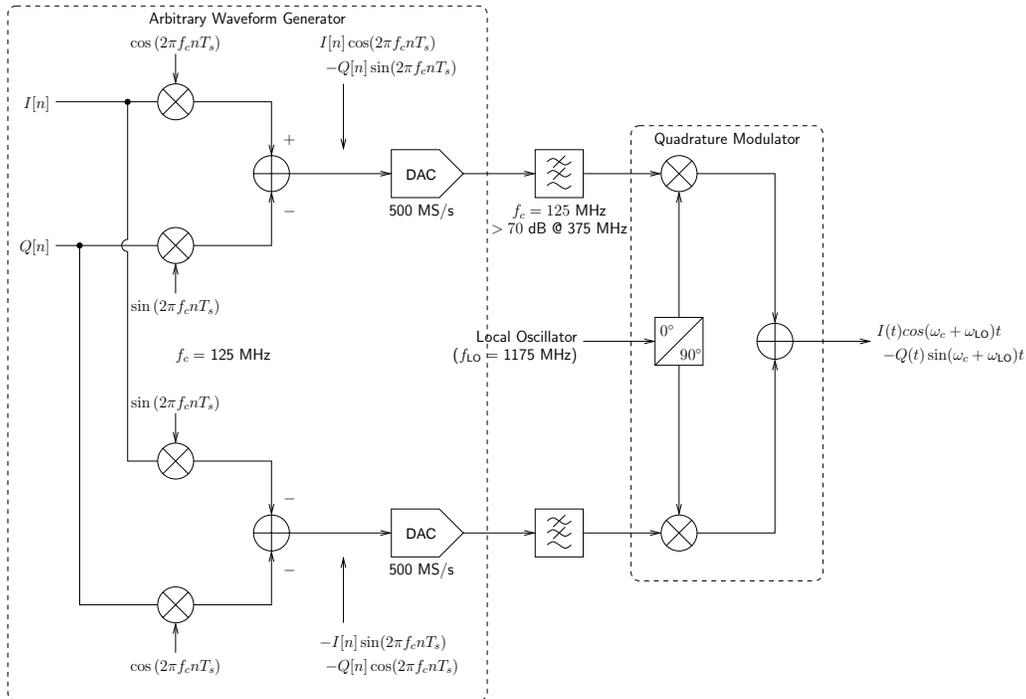
Figure 7: Waveform synthesis: baseband I and Q samples are digitally up-converted to 125 MHz. The analog output of the DACs are low-pass filtered and up-converted to 1300 MHz by a quadrature modulator.
