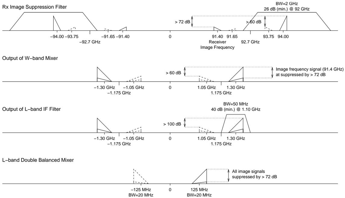
Figure 9: Down-conversion of the received signal. The first down-conversion stage converts the W-band received signal to L-band, and the second from L-band to the digital receiver intermediate frequency. Image-rejection mixers and filters are used to suppress unwanted image frequencies.
