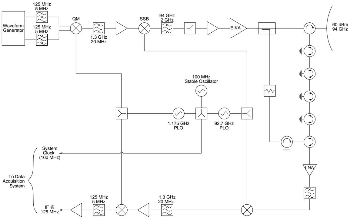
Figure 6: Block diagram of the single polarization HCR transceiver.
