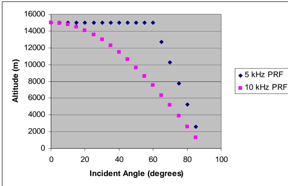
Figure 2: Maximum operating altitude as a function of incidence angle for 5 and 10 kHz.
