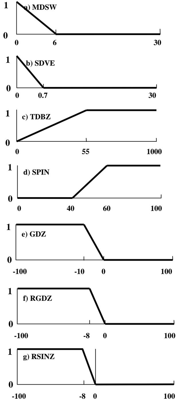
Figure 7. Membership functions for the sea clutter detection algorithm (SCDA) as used on the UAE EEC C-band radars.
