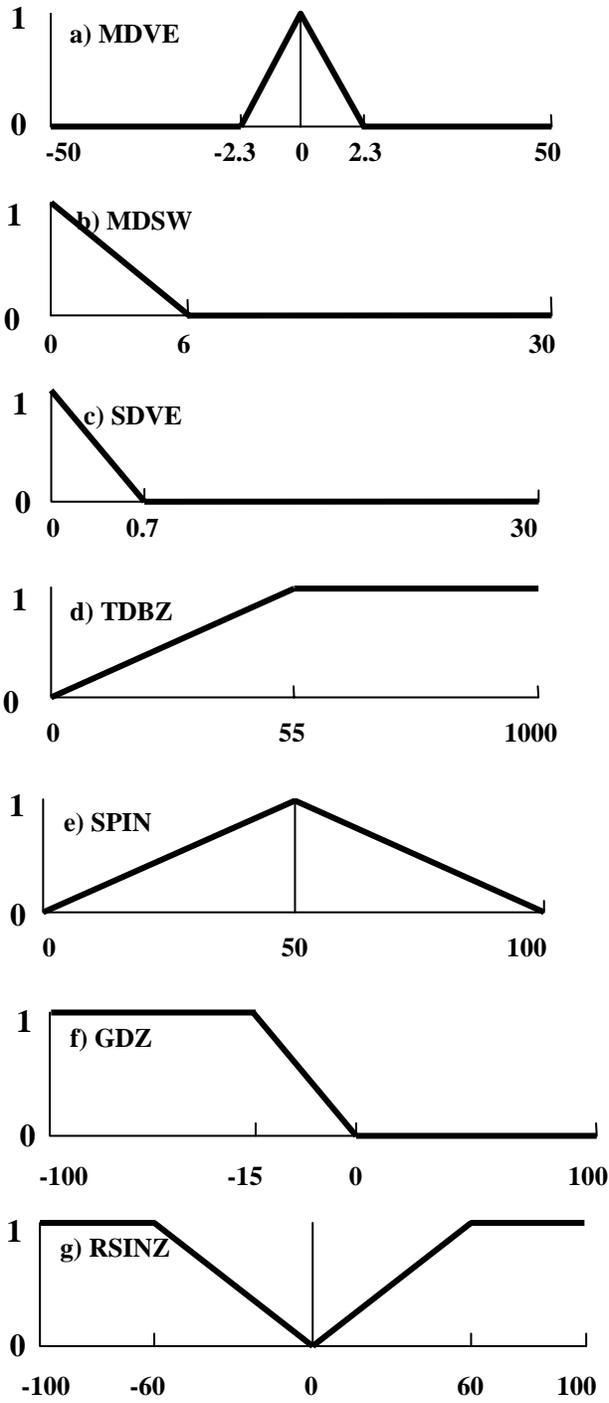
Figure 6. Membership functions for the modified AP clutter detection algorithm (mAPDA) as used on the UAE EEC C-band radars.
