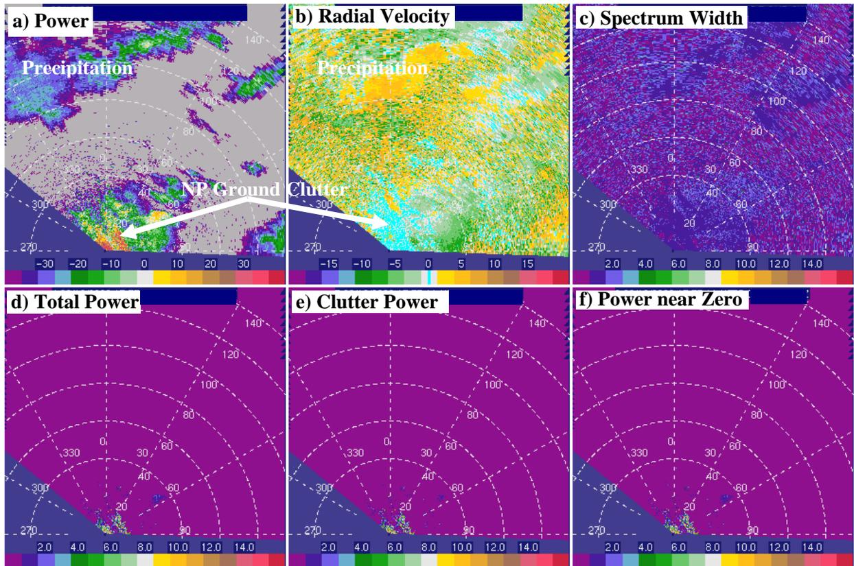
Figure 2. An example of spectral domain variables as calculated from KOUN time series data. Fields shown are a) reflectivity (dBZ), b) radial velocity ( $m s^{-1}$ ) with values near  $0 m s^{-1}$  shaded cyan, c) spectrum width ( $m s^{-1}$ ), d) the total power ( $P_{tot}$ ) field, e) the clutter power ( $C_p$ ) field and f) the power near zero ( $P_{nz}$ ) field. Notice the good discrimination between NP clutter and precipitation return.
