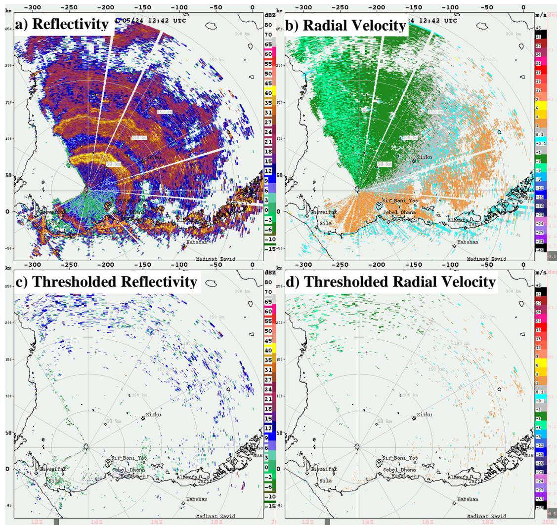
Figure 9. Radar data from the Dalma radar are shown from 24 May 2004 at 1242 UTC at 0.5 deg elevation. Fields shown are: a) unedited reflectivity (dBZ), b) unedited radial velocity (m/s), c) reflectivity data thresholded with the mAPDA and the SCDA (dBZ) and d) similarly thresholded radial velocity data (m/s). Radial velocity values near zero m/s are shaded cyan. Range rings are at 50 km intervals.
