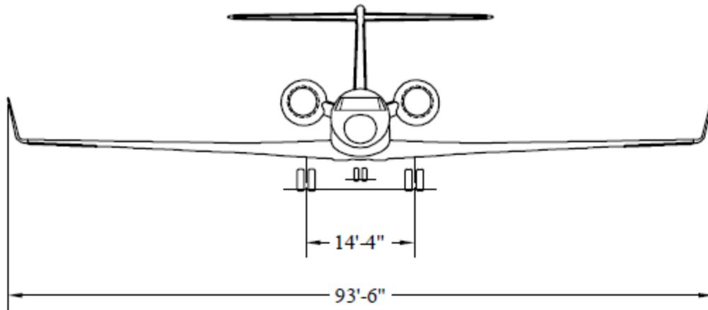
**Figure 2.1: Top, side and front dimensional views of the GV.**
