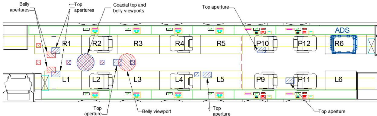
**Figure 2.2: GV cabin configuration. Floor stations P9-12 are emergency exits and can only contain seats. Floor stations L1, R1 and L6 can only contain racks. Stations P12 and R6 are permanently assigned to ADS and ADS operator.**
