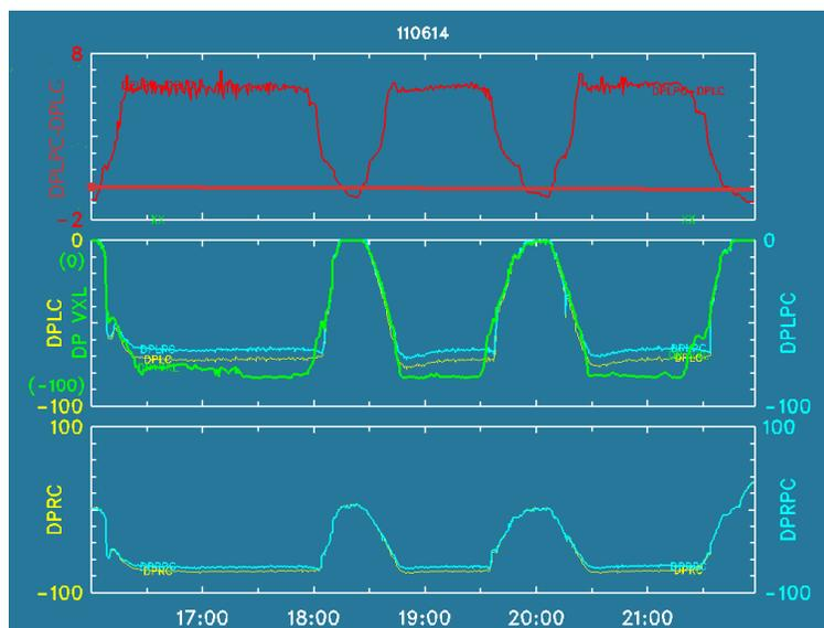
In this plot, the yellow traces in the bottom two plots are the original measurements, and the values corrected for housing pressure are shown in blue. The green trace in the second panel is the dew point from the VCSEL for the same time. The difference between the values of dew point for the left sensor is shown as the red trace in the top panel. The differences are often around 6°C and vary from -1 to +6 during the climbs and descents.
