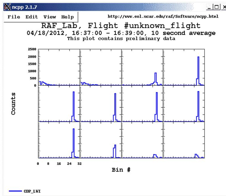
Figure 6: Apparent changes in measurement as droplet stream was moved ~0.3 mm, crossing the laser beam.
