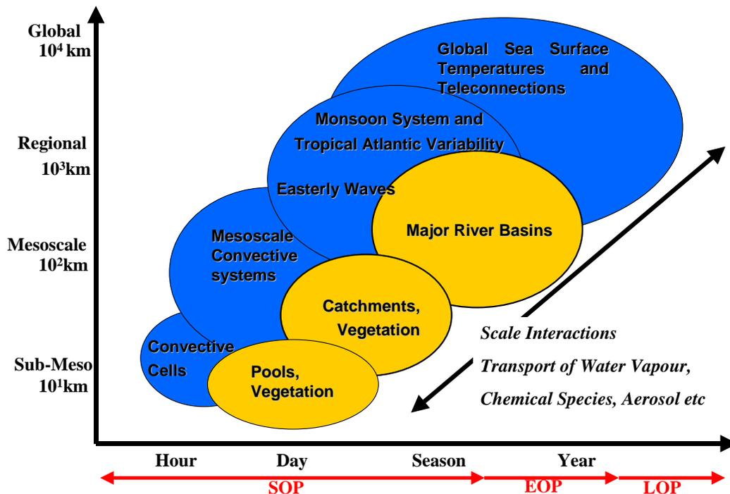
*Simplified schematic of key phenomena together with their associated space and time scales. The arrow is included to highlight the importance of scale interactions and transport processes in the WAM.*
