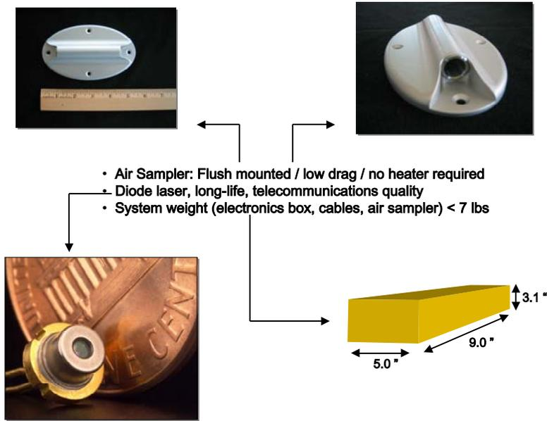
**Figure 7:** Composite of WVSS-II components
