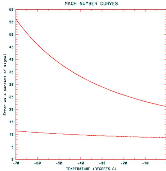
**Figure 2:** Error as a percent of signal for ambient RH. The random error of the RH sensor in the aircraft probe is assumed to be  $\pm 3\%$  (see text). The upper curve is for jet aircraft flying at  $M = 0.8$ . The lower curve is for a typical turboprop flying  $M = 0.45$ .
