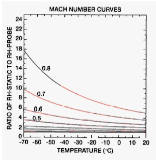
**Figure 1.** Ratio of  $RH_{\text{static}}$  to  $RH_{\text{probe}}$  as a function of temperature and Mach number. Mach number curves from 0.8 to 0.5 are labeled, the lower curves approach the value of 1.
