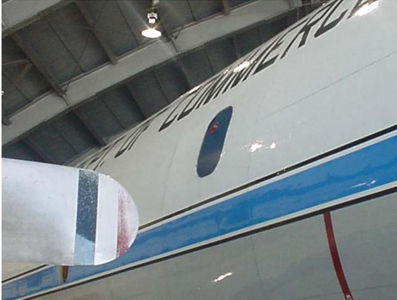
**Figure 4:** WVSS-II air sampler (red) mounted on blue window plate
