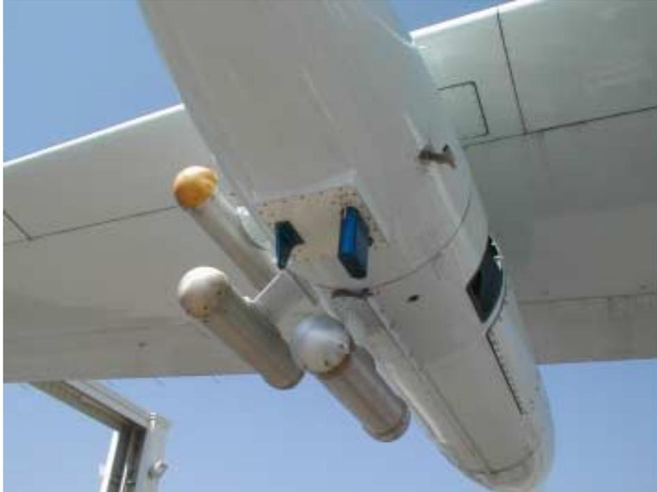
Figure 8. Picture of wing pod under the NCAR C-130 showing the “open path” diode laser (blue vertical extension in center of picture) and the WVSS-II (small probe located upper right from “open path” diode laser).
