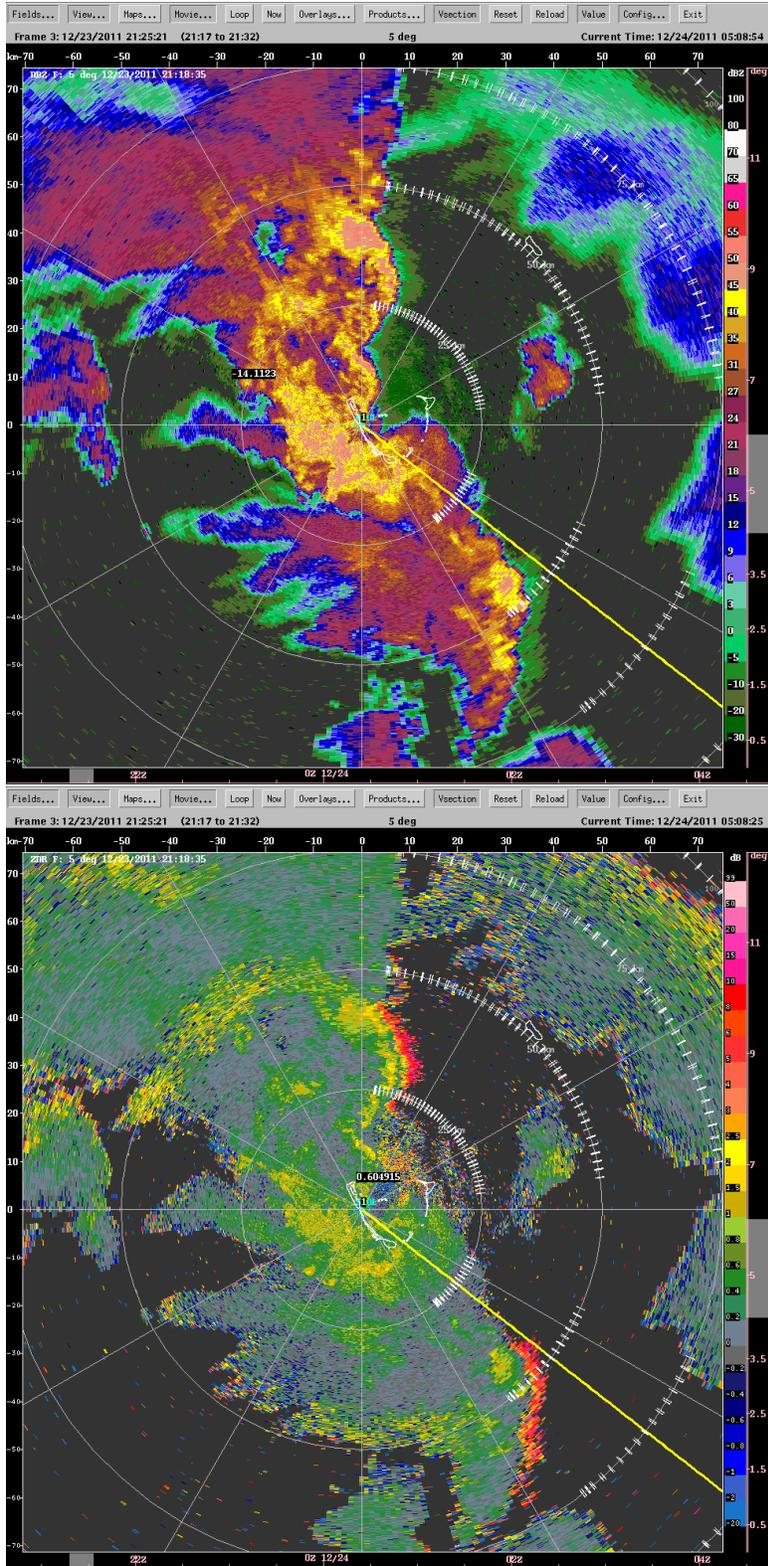
Figure 22: Sidelobe artifacts masquerading as biological scatter. The elevation angle is  $5^\circ$ .  $Z$ , top;  $Z_{dr}$ , bottom. Biological scatter is not likely at these higher elevation. The high  $Z_{dr}$ s (red/pink colors) are due to non-matched H and V antenna pattern sidelobes.
