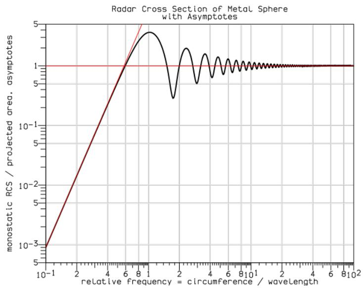
Figure 20: Back scatter cross section for spheres.
