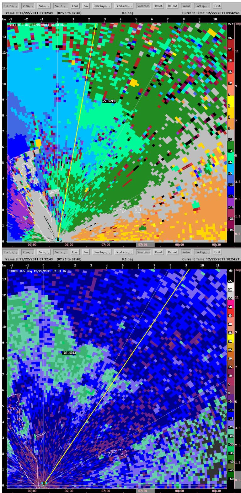
Figure 9: Sea clutter mixed with weather example. Velocity, top, *LDR* bottom.
