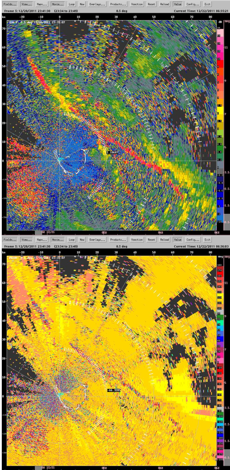
Figure 14: Bird echoes.  $Z_{dr}$ , top,  $\phi_{dp}$  bottom. Note the noisy  $\phi_{dp}$  along the bird-line cause by Mie scattering.
