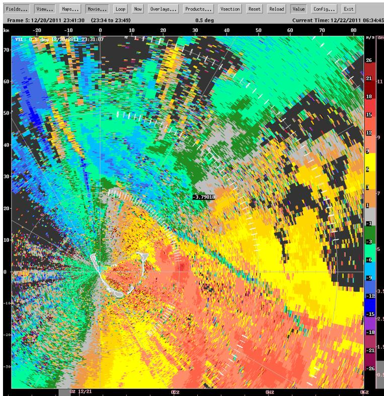
Figure 15: Bird echoes, radial velocity. Birds are flying against the wind at about 20 MPH. Bugs can not do this.
