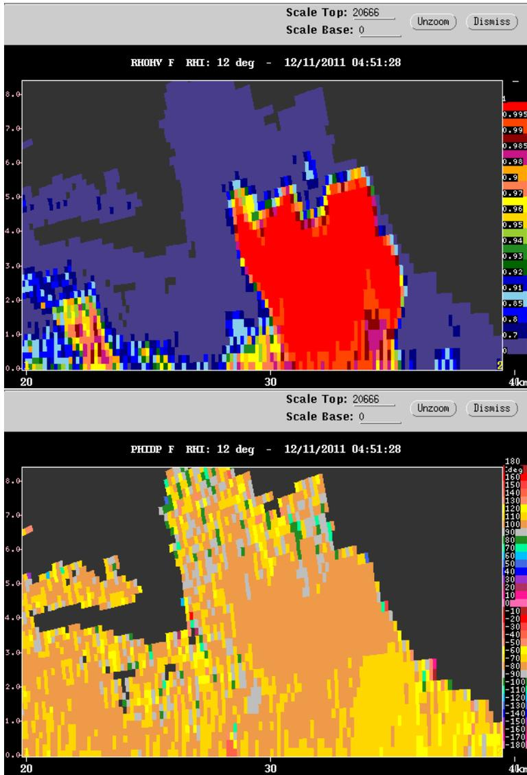
Figure 26: Three-body scattering.  $\rho_{hv}$ , top,  $\phi_{dp}$  bottom.
