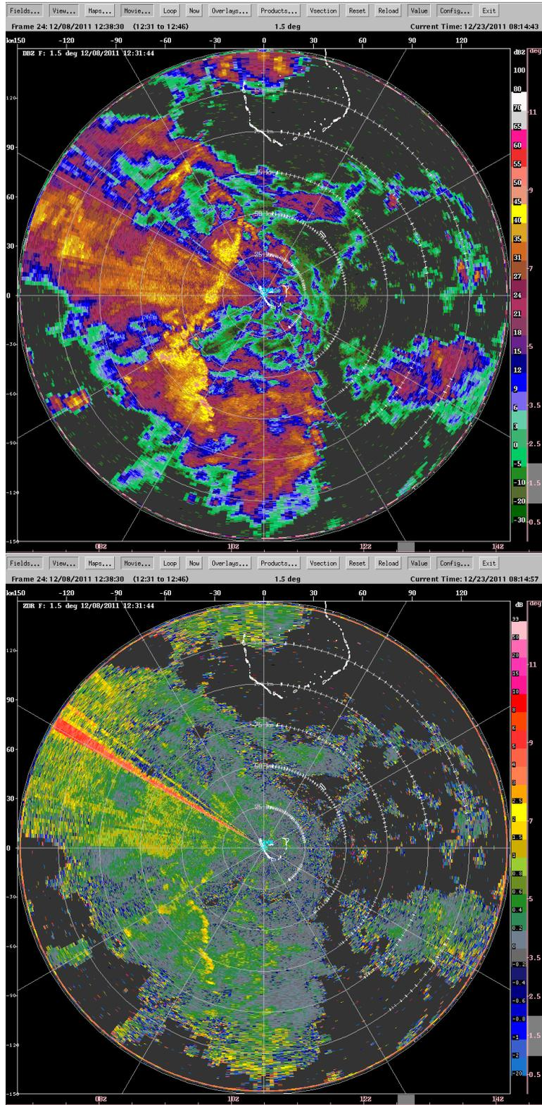
Figure 23: The high  $Z_{dr}$  streak to the north-west is due to differential attenuation/scattering by the tower close to the radar shown in Fig. 24. The streak is only seen when there is precipitation echo in that radial.
