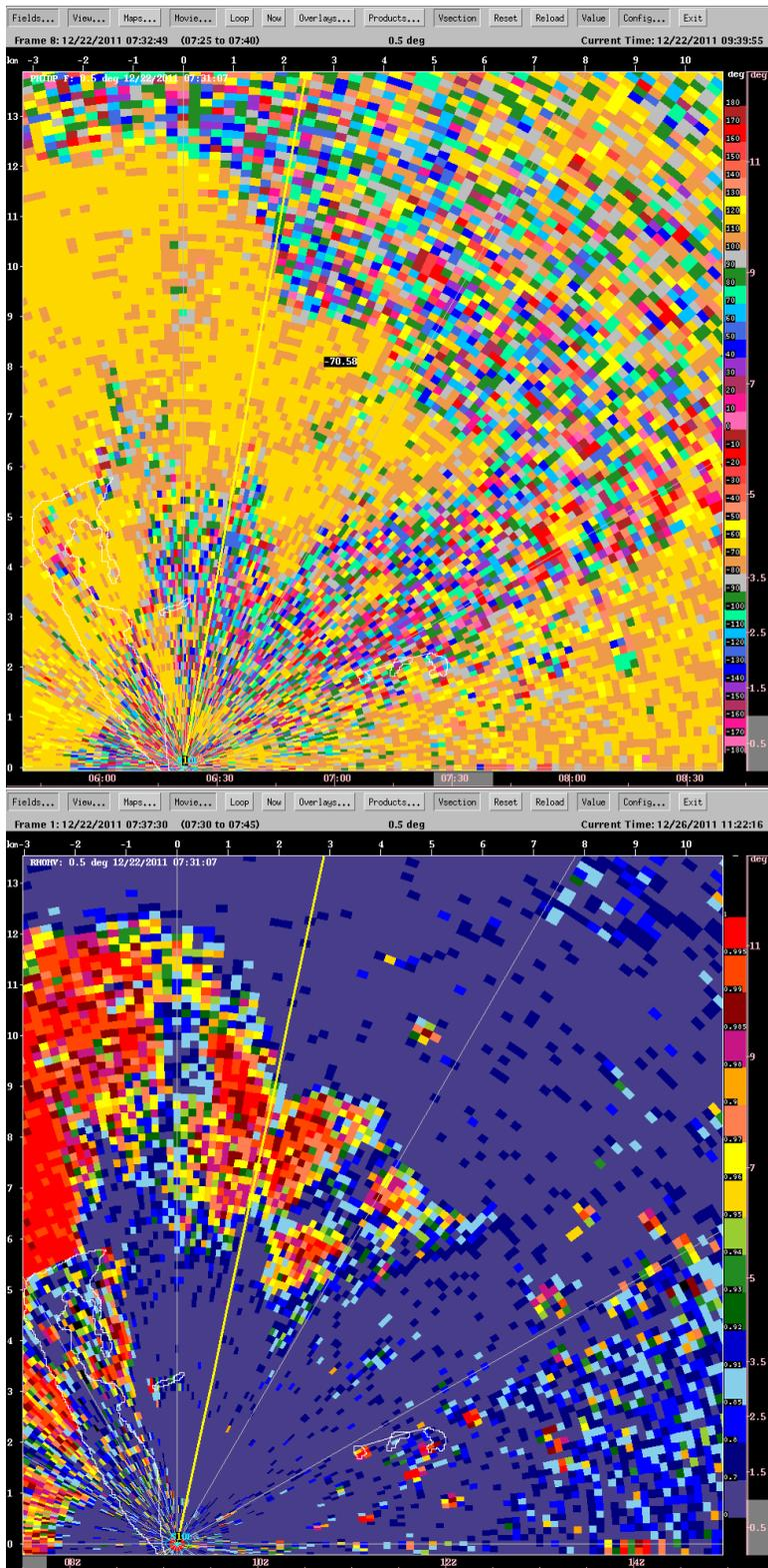
Figure 8: Sea clutter mixed with weather example.  $\phi_{dp}$  top,  $\rho_{hv}$  bottom.
