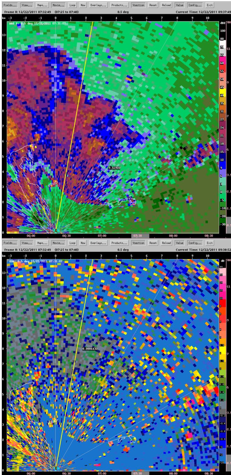
Figure 7: Sea clutter mixed with weather example.  $Z$  top,  $Z_{dr}$  bottom.
