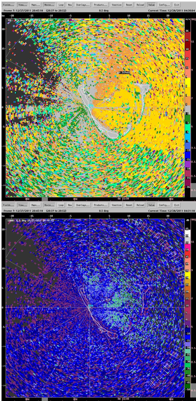
Figure 6: Sea clutter night time example. Velocity, top, *LDR* bottom.
