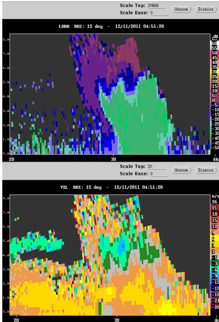
Figure 27: Three-body scattering. *LDR*, top. Velocity, bottom.
