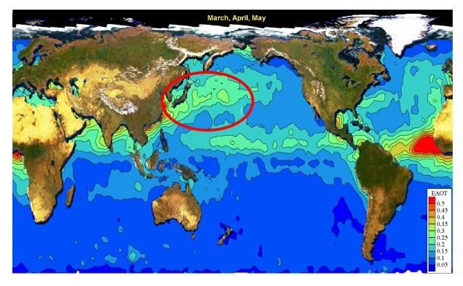
Aerosol optical depth over the oceans as measured by AVHRR. The red circle shows the plume from the Asian continent that will be studied in ACE-Asia (figure from R. Husar)
