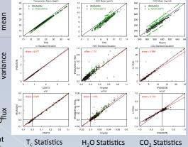
Example of nighttime fluxes: The correlation coefficient between w and CO<sub>2</sub> is 30% lower from the LI-7500, presumably due to path separation. Our model of this separation predicts only a 4% effect, so even corrected fluxes would be underestimated.
