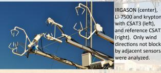
CO<sub>2</sub> density changes due to changing temperature and to changing CO<sub>2</sub> mixing ratio. After removing the air density change, fluxes are more realistic from IRGASON (center), the IRGASON, with CO<sub>2</sub> uptake during the day. This LI-7500 and krypton implies that our LI-7500 was not well calibrated. with CSAT3 (left), and reference CSAT3 (right). Only wind
