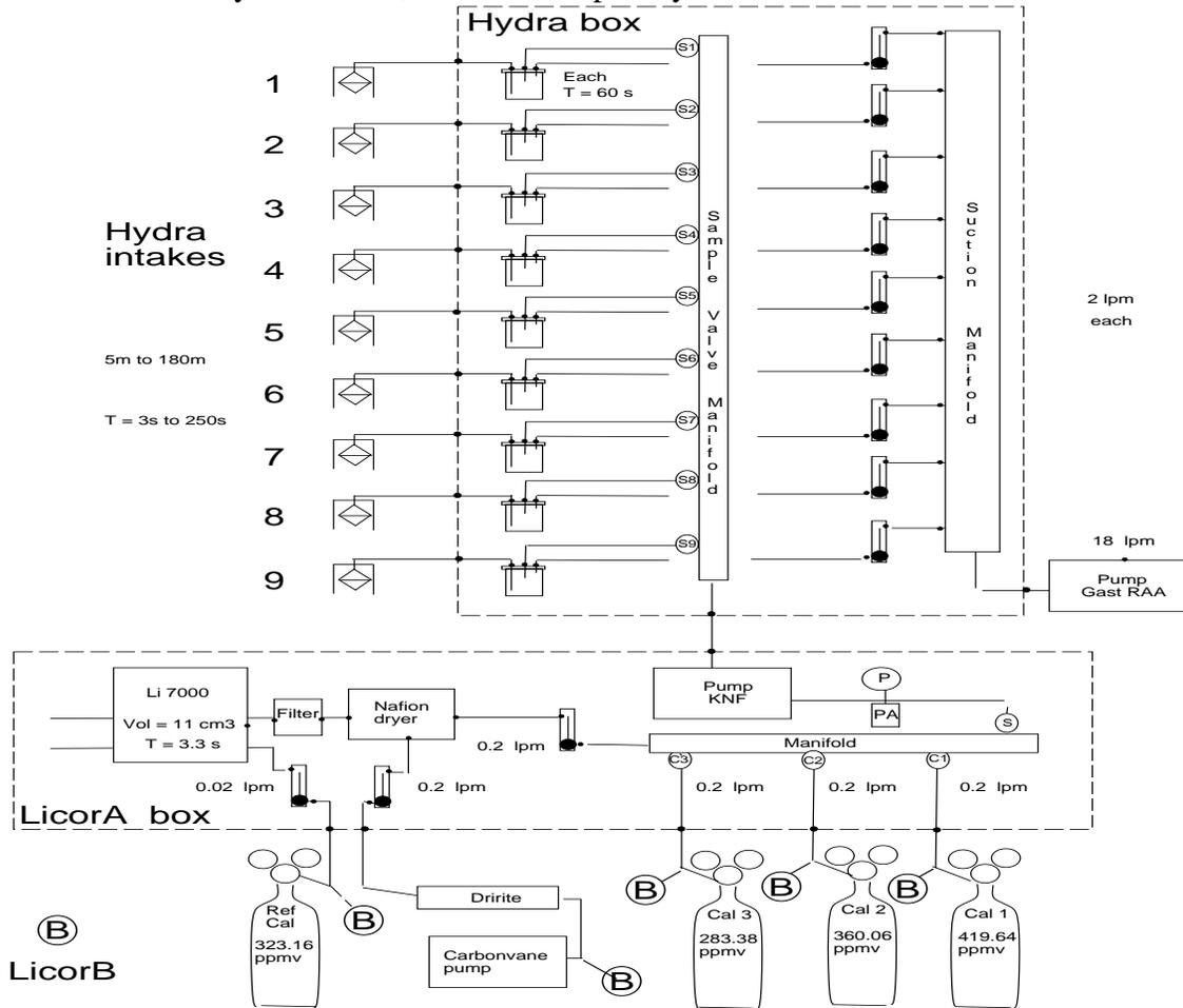
The Hydra is essentially a duplex system with two sets of nine sample air streams supplying two separate Licor 7000 closed path infrared absorption CO<sub>2</sub> analyzers. The designation used is Hydra/Licor A and Hydra/Licor B. Each of the two systems is represented by the above schematic.
