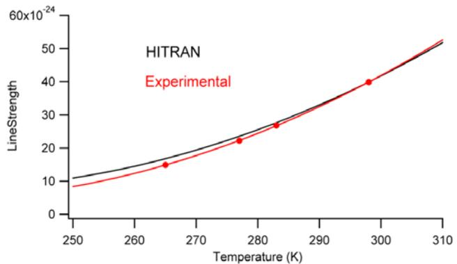
**Figure 4** Comparison of HITRAN and experimentally determined linestrength from cold bath measurements at atmospheric pressure.
