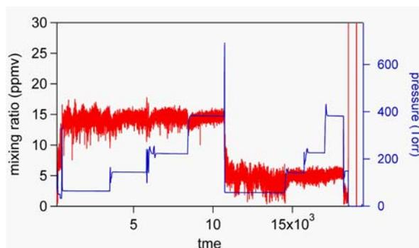
**Figure 5** Measured concentration as pressure varies at constant mixing ratio. The mixing ratio is changed halfway through the data set.
