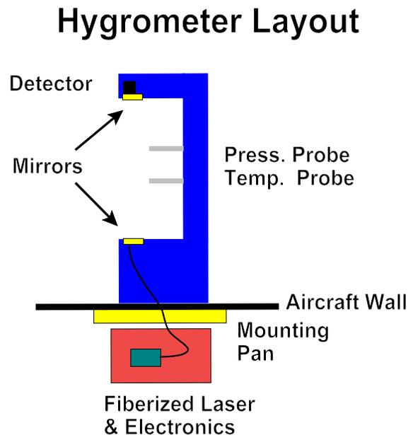
**Figure 2** Instrument schematic
