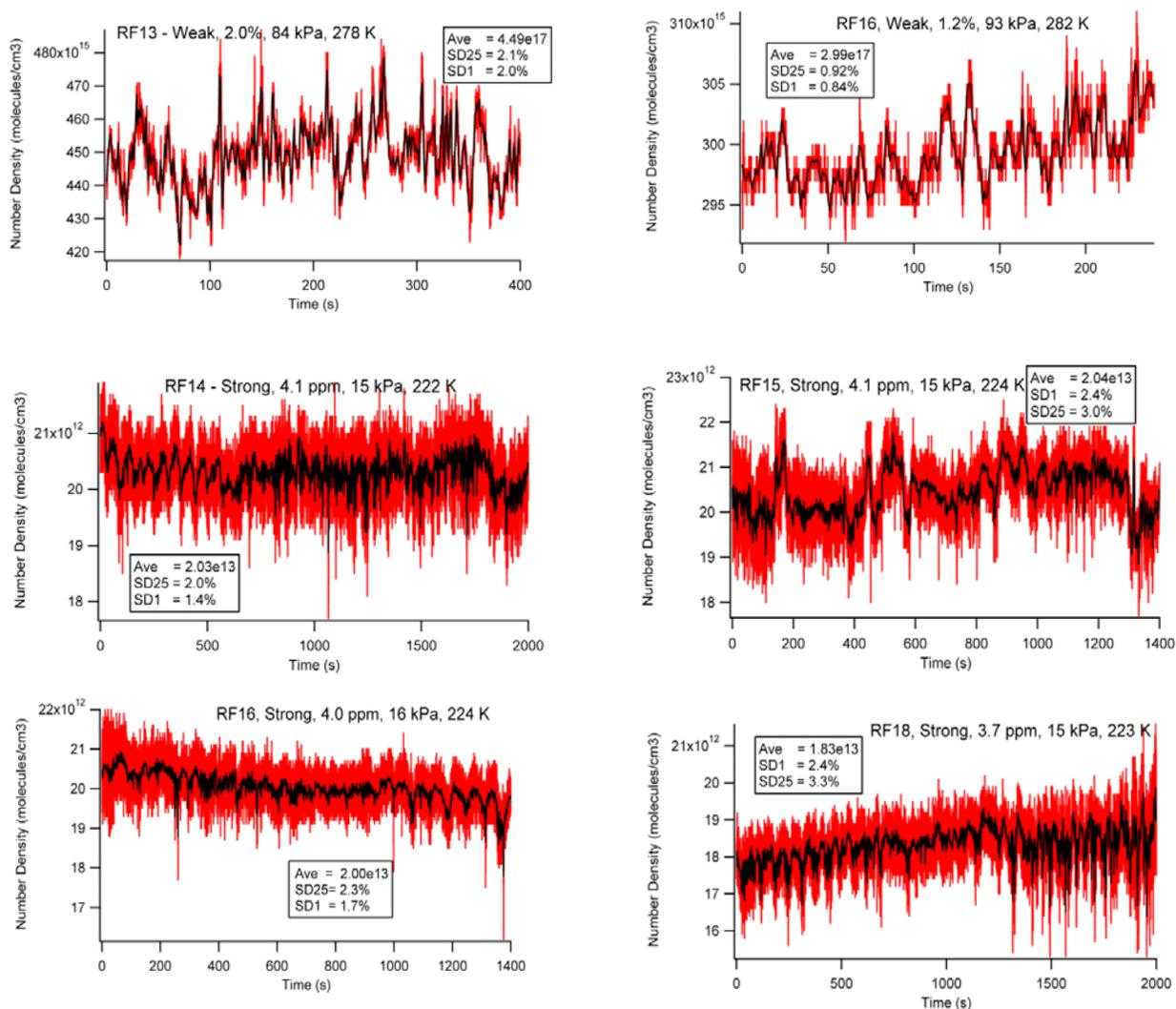
**Figure 7** Noise assessment during later START08 research flights. The measurement mode (strong or weak), the water vapor concentration, pressure, temperature, and research flight number are noted. The red curves are the 25 Hz data and the black curves are the 1 second averaged data. In the box, the average concentration is shown along with the standard deviation for 1 Hz averaged data and the normal 25 Hz data. No trend analysis has been applied in determining these statistics.
