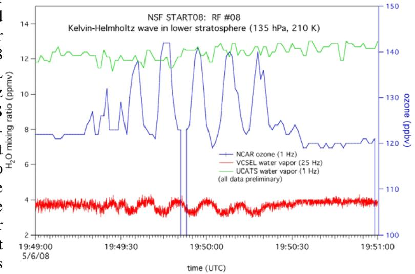
**Figure 8** Kelvin-Helmholtz waves during RF #08 for VCSEL (red) and UCATS water vapor (green) and NCAR ozone (blue). The absolute differences between the UCATS and VCSEL were typical for the first deployment.
