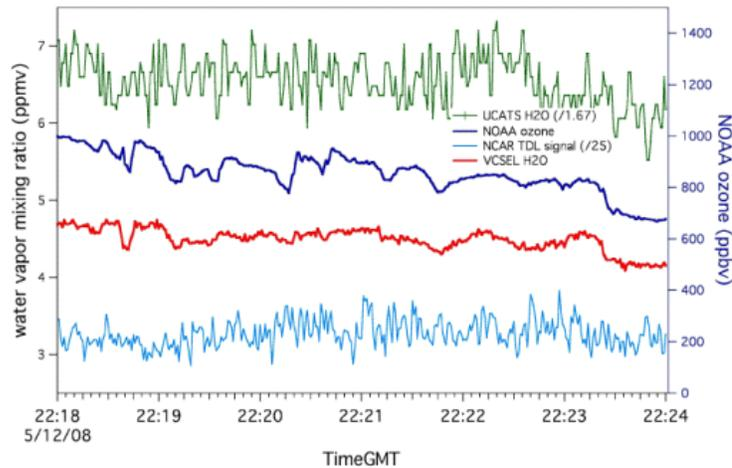
**Figure 9** VCSEL, UCATS H<sub>2</sub>O, and NCAR TDL preliminary data for lower stratospheric conditions (133 hPa, 223 K) during RF #10. The VCSEL shows correlations with ozone during this leg (blue, right axis) that are not captured by the other laser hygrometers.
