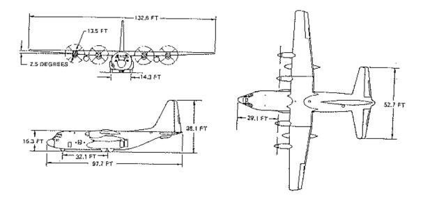
. Figure 1.2 Three views of the C-130Q aircraft
