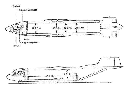
Figure 1.3 C-130Q fuselage cross section.
