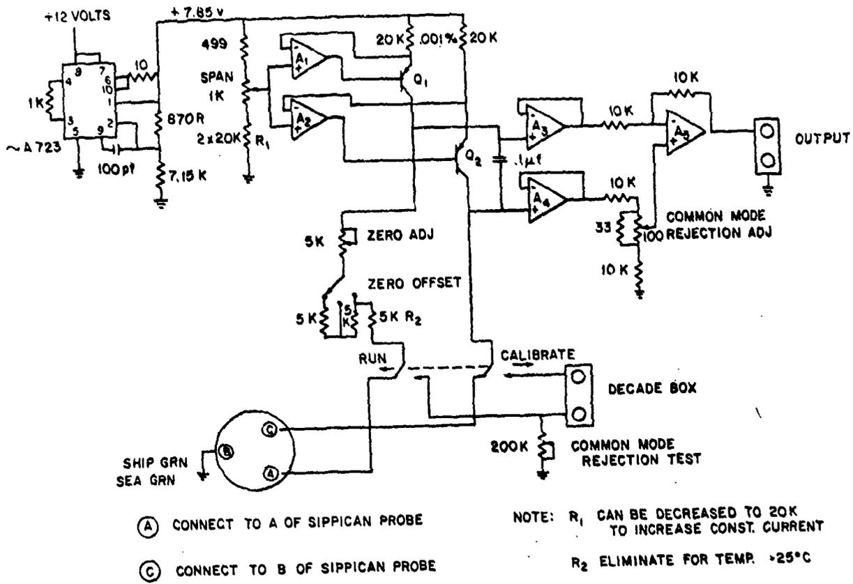
Figure 22. Electric circuit diagram of the EXBT system.
