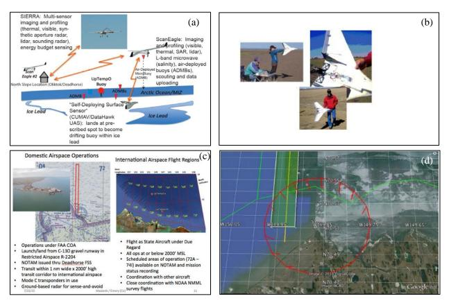
*Figure 2* (a) *MIZOPEX* concept of operations; (b) Datahawk UAS; (c) planned airspace over domestic and international waters; (d) zoomed view of restricted airspace at Oliktok Point and corridor to international waters.
