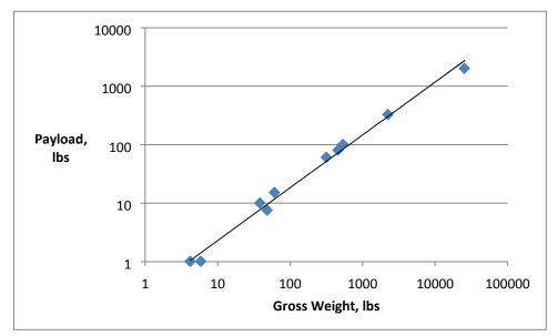
Payload is proportional to vehicle gross weight as shown in the following Figure 2.
