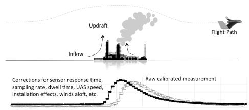
*Figure 10.* Sample data correction of an in situ gas measurement correcting for sensor, integration, and flight path issues.
