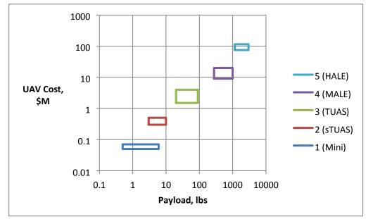
Figure 4. Vehicle Cost and payload capacity ranges for DoD UAV Groups (compiled from various public domain sources).
