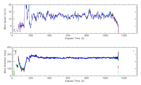
*Figure 8.* Wind speed (top) and wind direction (bottom) from the Rain Dynamics wind sensing system. In the first three minutes of the time series the sensor is acquiring a GPS lock and these data are rejected.
