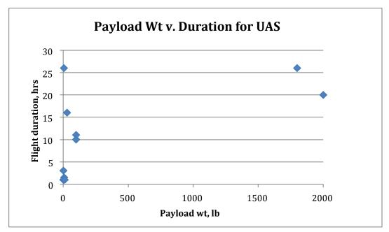
Figure 7. Payload / flight duration regime of current UAS
