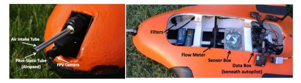
Figure 9. Sample gas sensing system with integrated environmental sensors including CO<sub>2</sub> & CH<sub>4</sub>.
