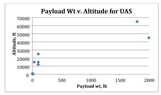
Figure 6. Payload / altitude regime of current UAS
