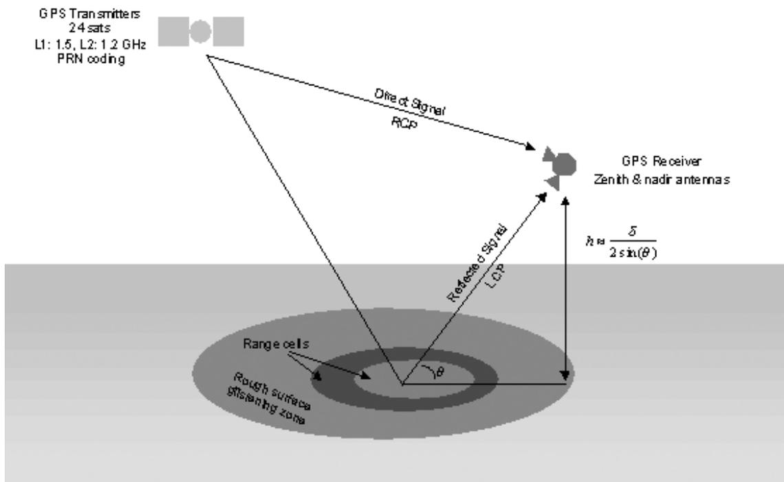
Figure 22. Bistatic radar configuration of reflected GPS signals.
