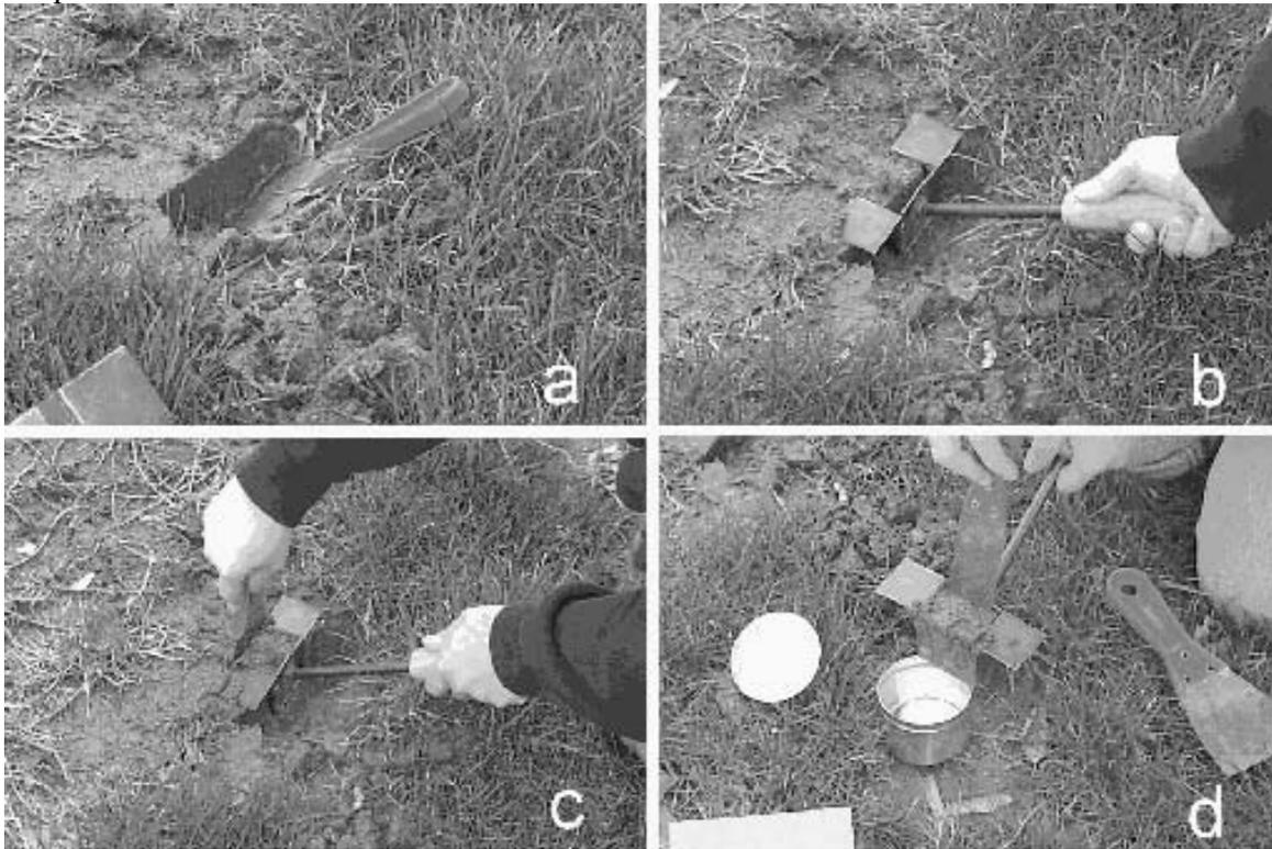
Figure P7. How to take a gravimetric soil moisture sample.
