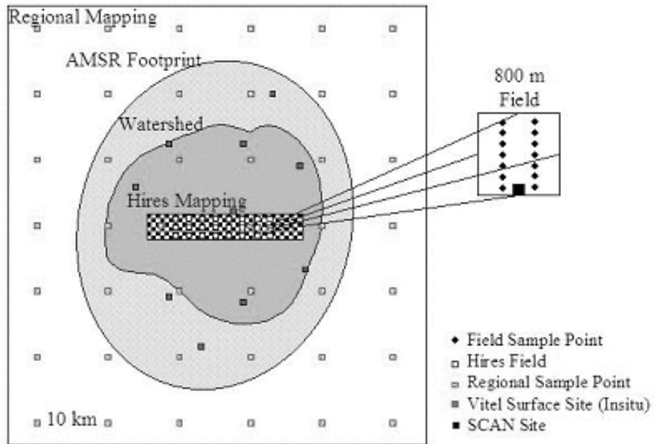
Figure 25. The general approach used in SMEX04 soil moisture sampling.
