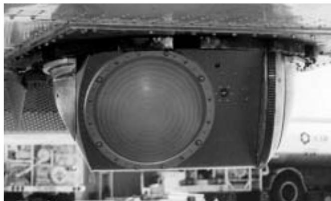
Figure 18. PSR/C scanhead installed on the NASA P3-B aircraft during the SGP99 experiment.
