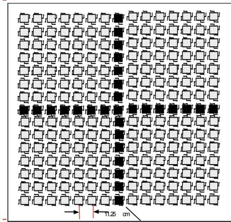
Figure 20. Antenna patch array shown configured for measuring using a cross “+” configuration.
