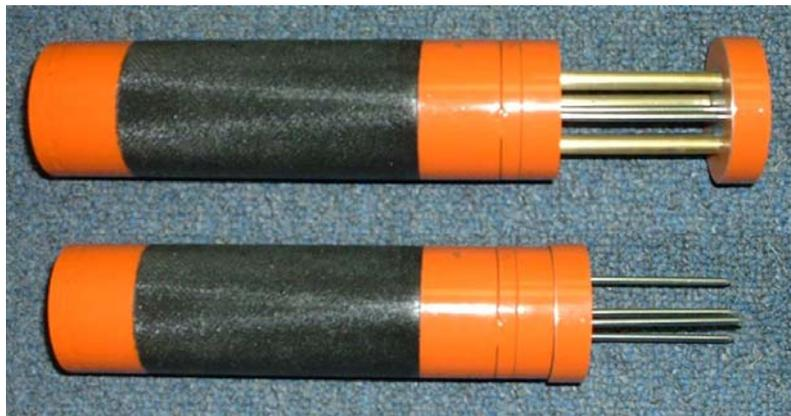
Figure P5: SMITY, Soil Moisture Insertion Tool, with slider extended and retracted.
