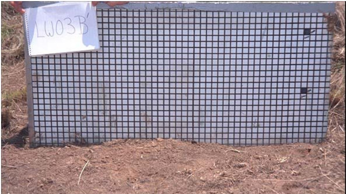
Figure P14. Surface roughness photo.
