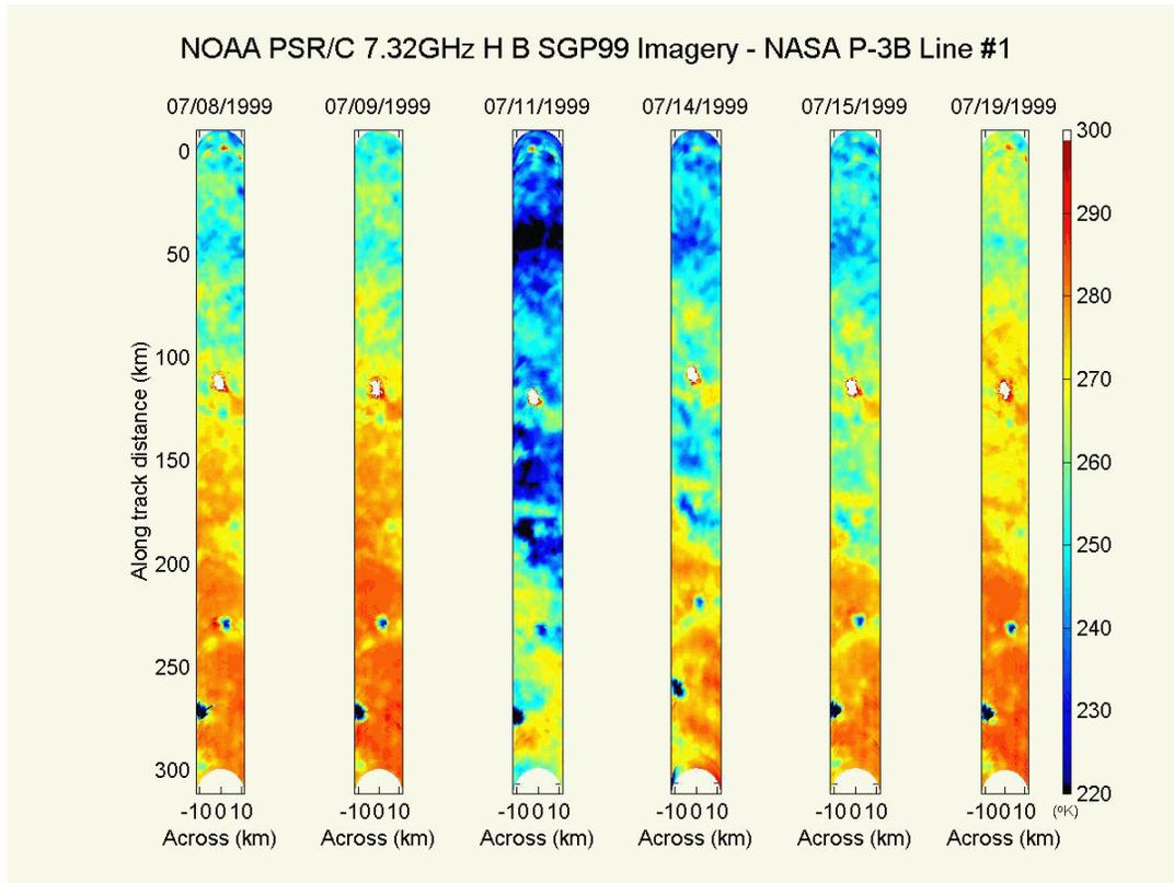
Figure 19. SGP99 PSR/C conically-scanned brightness temperature imagery 7.325 GHz channel, H-polarization, North looking.
