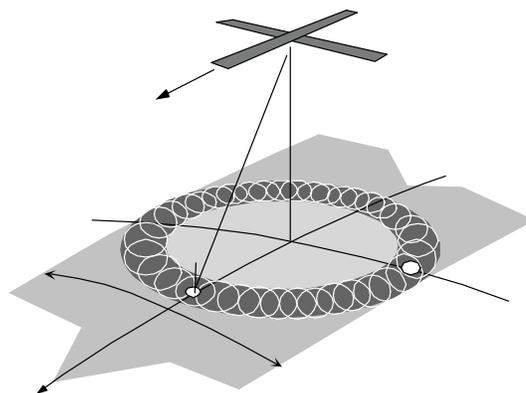
Figure 21. A thinned array in a nadir-pointing mode illustrating the potential for conical scanning.
