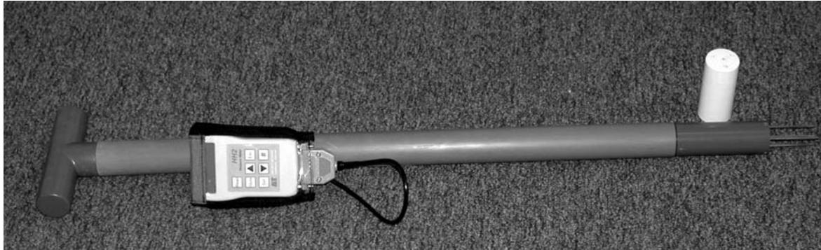
Figure P2. Theta Probe Type 1 (with extension rod).
