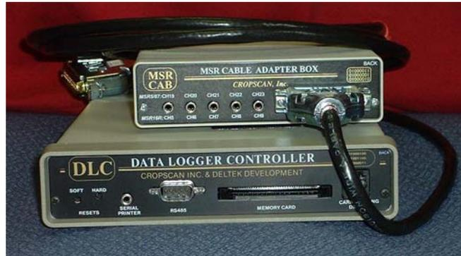
Figure P17. Data logger controller and cable adapter box.
