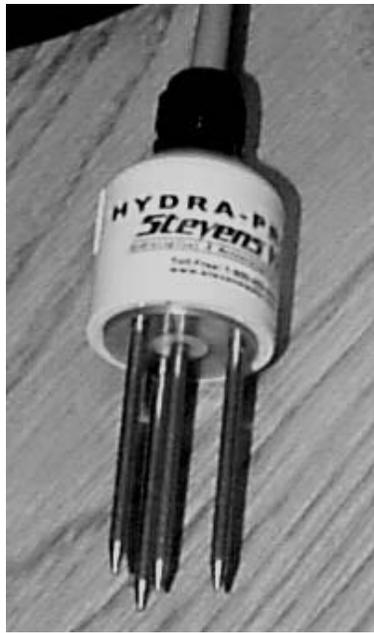
Figure P11. The Hydra probe used at the tower locations.
