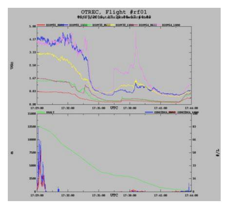
Figure A1. Time series from OTREC RF01. Upper box shows diode voltages for the 25-micron probe (LWOO) (generally large values), and from the 10-micron probe (RWOI) (generally smaller voltages). Bottom box shows altitude and concentrations of all particles from the two probes.
