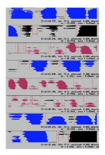
Figure A4. Particle images from 17:43:25. Red particles are from the 25-micron probe (LWOO), and blue particles are from the 10-micron probe (RWOI). These particle images should show solid round raindrops; instead the images have missing horizontal stripes and ragged edges where diodes are not triggering (likely due to condensation). These images are considered bad, and they should not be used for analysis.
