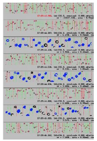
Figure A2. Particle images from 17:29:44. Red particles are from the 25-micron probe (LWOO), and blue particles are from the 10-micron probe (RWOI). These particle images are considered good. The blue particles are collected from a 640-micron wide section, and the red images are collected from a 1600 micron wide section.
