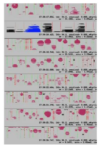
Figure A3. Particle images from 17:38:20. Red particles are from the 25-micron probe (LWOO), and blue particles are from the 10-micron probe (RWOI). These particle images should show solid round raindrops; instead the images have missing horizontal stripes and ragged edges where diodes are not triggering (likely due to condensation). These images are considered bad, and they should not be used for analysis.
