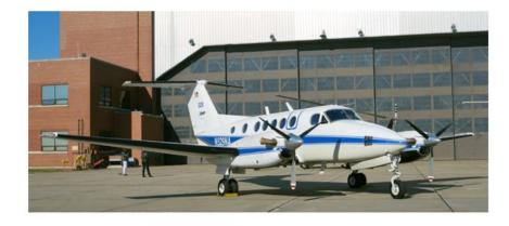
The KingAir B-200 aircraft, owned and operated by NASA with funding from DOE, has a downwardpointing LIDAR that will measure the concentrations and properties of aerosols below its flight altitude.
