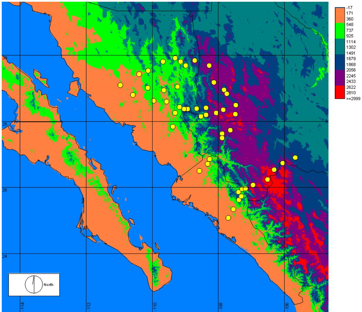
**Figure 2. Map of PHASE 1 raingages overlain topography separated by elevation bands. Shading color indicates elevation band: Orange (Band 1), Light Green (Band 2), Aqua (Band 3), Blue (Band 4), Purple (Band 5), Red (Band 6). Note the distinct lack of terrain in elevation Band 3 along the western Sierra Madre Occidental.**
