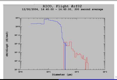
Needed Measurements Examples of Measured Hydrometeor Size Distributions
