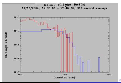
Needed Measurements Examples of Measured Hydrometeor Size Distributions
