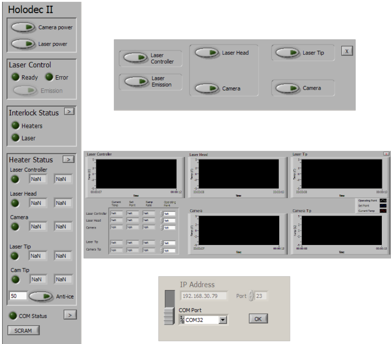
Figure 6.2: Holodec Control front panel (far left) with subpanels. The top pane in the front panel controls and indicates power to the laser and camera. The "Laser Control" pane shows the status of the laser and provides the switch to start laser emission when the laser is in the "ready" state. The Interlock Status pane indicates the status of the interlocks with the option to open a subpanel for more granular control. The Heater Status pane shows the current temperature and operating point for the five managed channels as well as an status indicator light. The anti-ice button at the bottom of the pane toggles the anti-ice mode which elevates the temperature of the instrument tips to the specified temperature (default 50C). This panel also has the option to open a subpanel which shows historic temperature data and includes the ability to alter the operating point of individual channels. At the bottom of the front panel is a com status light that indicates the status of the connection to the instrument and a button to open the com settings subpanel. The SCRAM button provides an emergency shutdown mechanism which opens all interlocks and kills power to the laser and camera.
