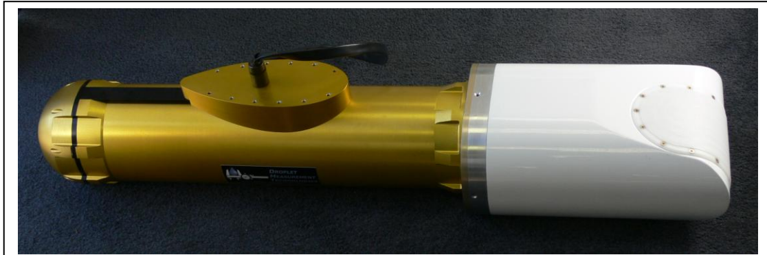
Figure 3-1. HIAPER MTP fairing (white), DMT canister (gold) and HDPE window (white).
