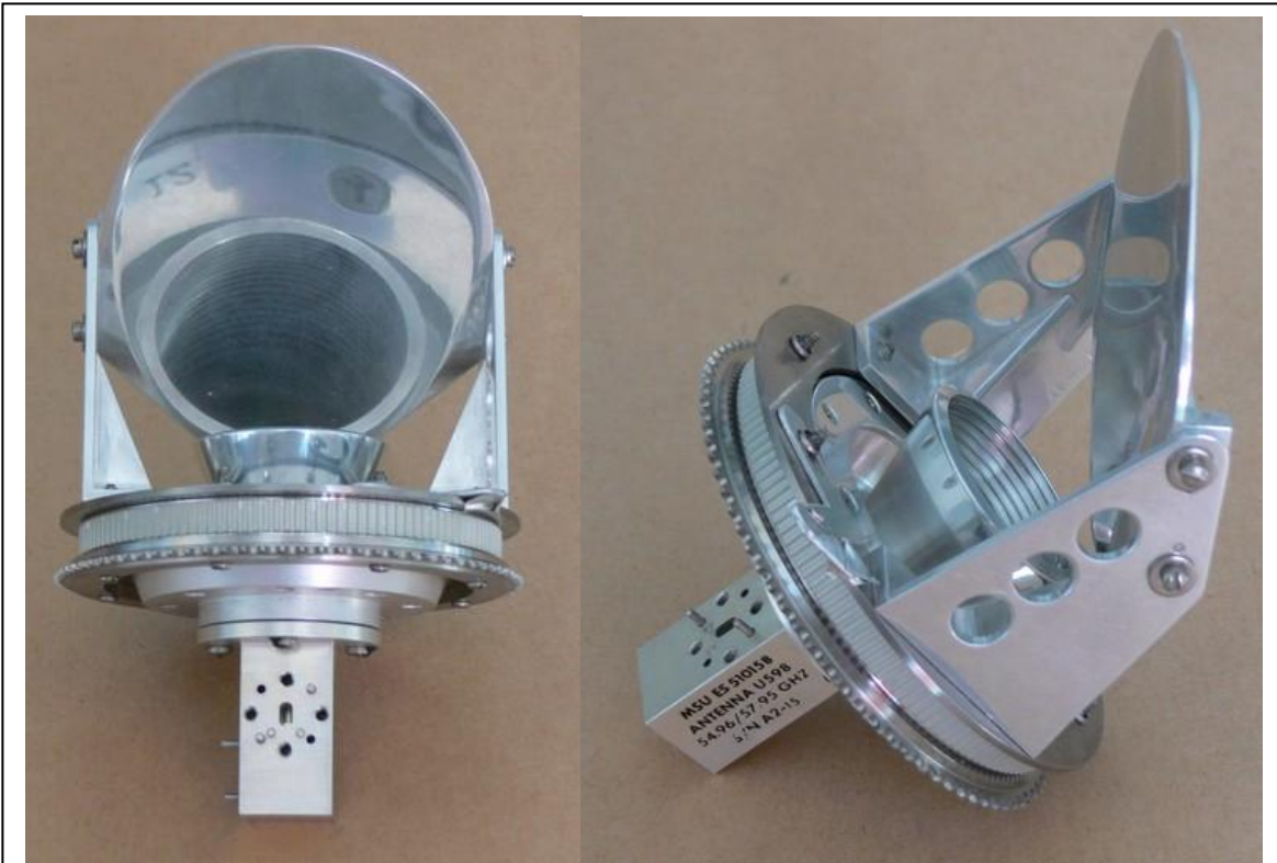
Figure 3-5. Scan mirror, corrugated feed horn, chain drive, and orthomode transducer. Note that the sprocket for the chain drive is mounted outside of the original belt drive sprocket. This was done so that the reference target could be mounted closer to the antenna. Previously, it was mounted in place of the original belt drive sprocket.
