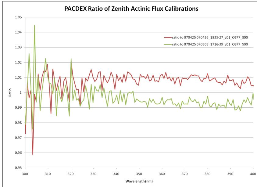
The figure below shows the ratio of two irradiance calibrations performed near the beginning and end of PACDEX with the absolute differences <2% through most of the spectrum. High noise is seen where the instrumentation sensitivities and/or lamp output are lowest. The high values around 1400 and 1900 nm are the results of changes in water vapor in the calibration air surrounding the calibration stand.
