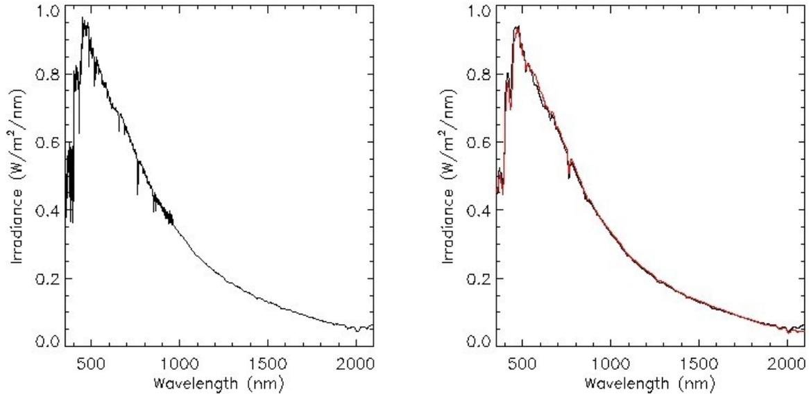
The absolute accuracy depends largely on the accuracy of the calibration standard. The NIST standards are rated at 2% in the visible and 5-6% in the NIR (2000 nm).
