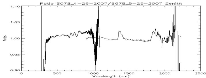
The wavelength calibration reproducibility of <0.02 nm translates into an uncertainty of 1.0% in the UV-B and 0.5% in the UV-A and visible for the actinic flux and negligible error for the irradiance.
