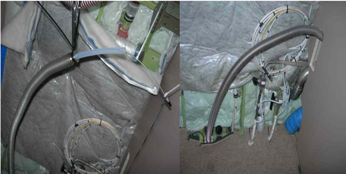
Zenith Fiber: Bare fiber entering cabin, Routed behind galley to protect fiber union
