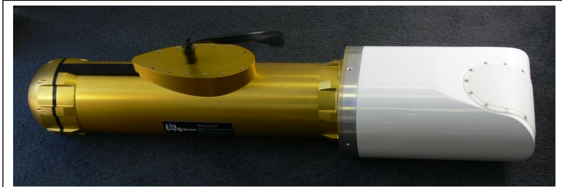
Figure 3-1. HIAPER MTP fairing (white), DMT canister (gold) and HDPE window (white). The HALO MTP will use a custom composite canister carrier ( Figure 1-5 )
