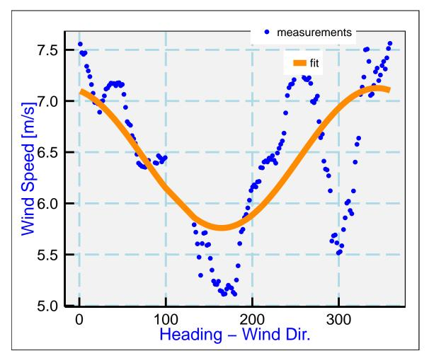
Figure 9: Measured wind speed from the left-turn circles in the circle pattern shown in Fig. 5, as a function of the difference between the heading and the mean wind direction.
