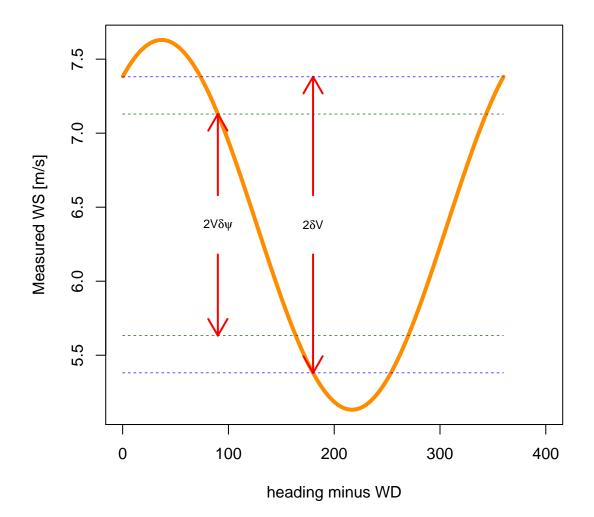
Figure 8: Predicted dependence of measured wind speed on direction of flight relative to the wind direction, for assumed errors of  $\delta V = 1$  m/s and  $\delta \psi = 0.3^{\circ}$ .
