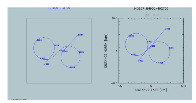
Figure 5: Example of circle flight pattern, FRAPPE flight 9, 19:19–19:27 UTC. Left side: normal flight track; right side, flight track plotted in a reference frame drifting with the horizontal wind.
