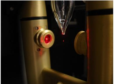
Figure 1. Photo shows droplet stream illuminated in CDP laser beam. Droplet is embedded in steady air stream accelerated and focused in glass nozzle.
