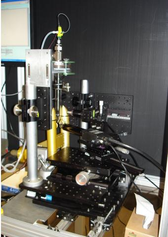
Figure 2. Test apparatus holds CDP (gold) fixed in place. Droplet stream and air flow downward through CDP laser beam. X/Y/Z micro-positioner stages support the droplet generator and two cameras. Movement is along and perpendicular to the laser beam.
