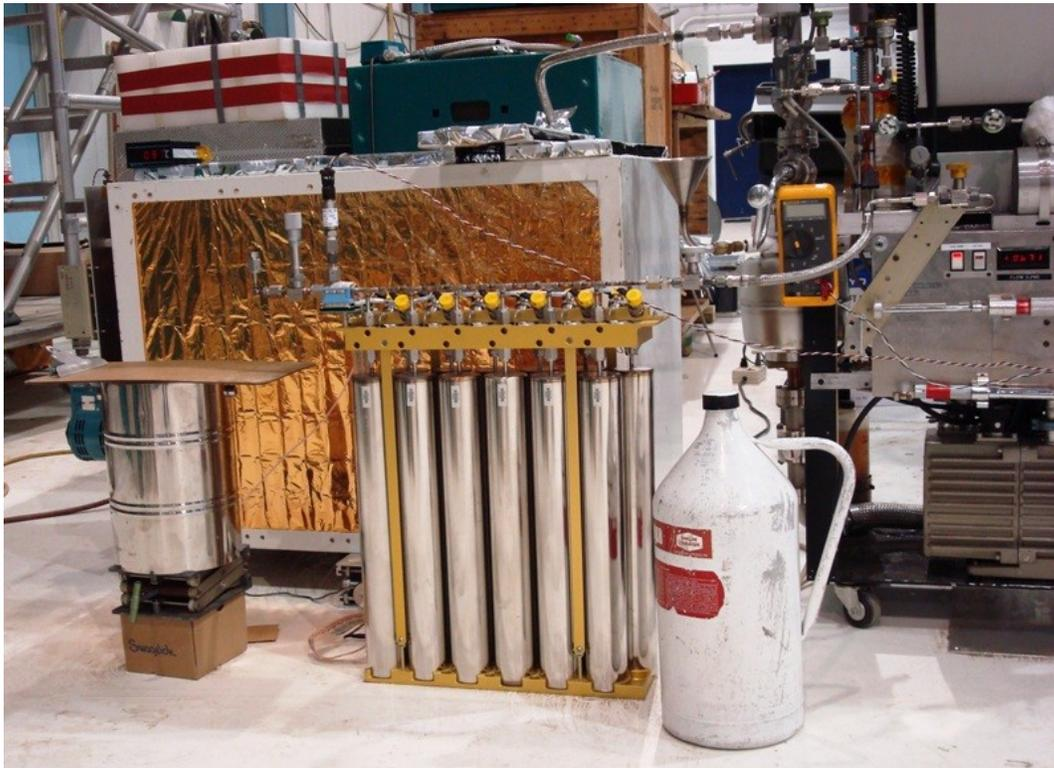
**Figure A2.** Bakeout system used to prepare AWAS module sampling. Also shown is part of the system used to transfer air from AWAS canisters to individual canisters.
