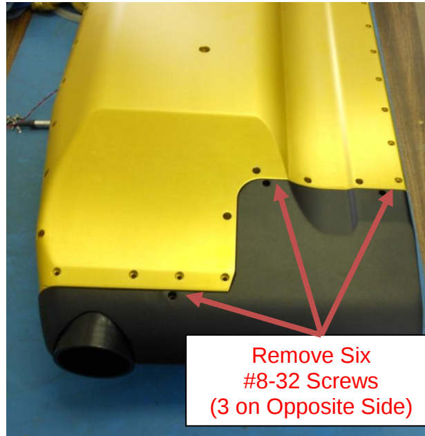
Figure 6.4.1: Screw locations for fairing removal required for purging
