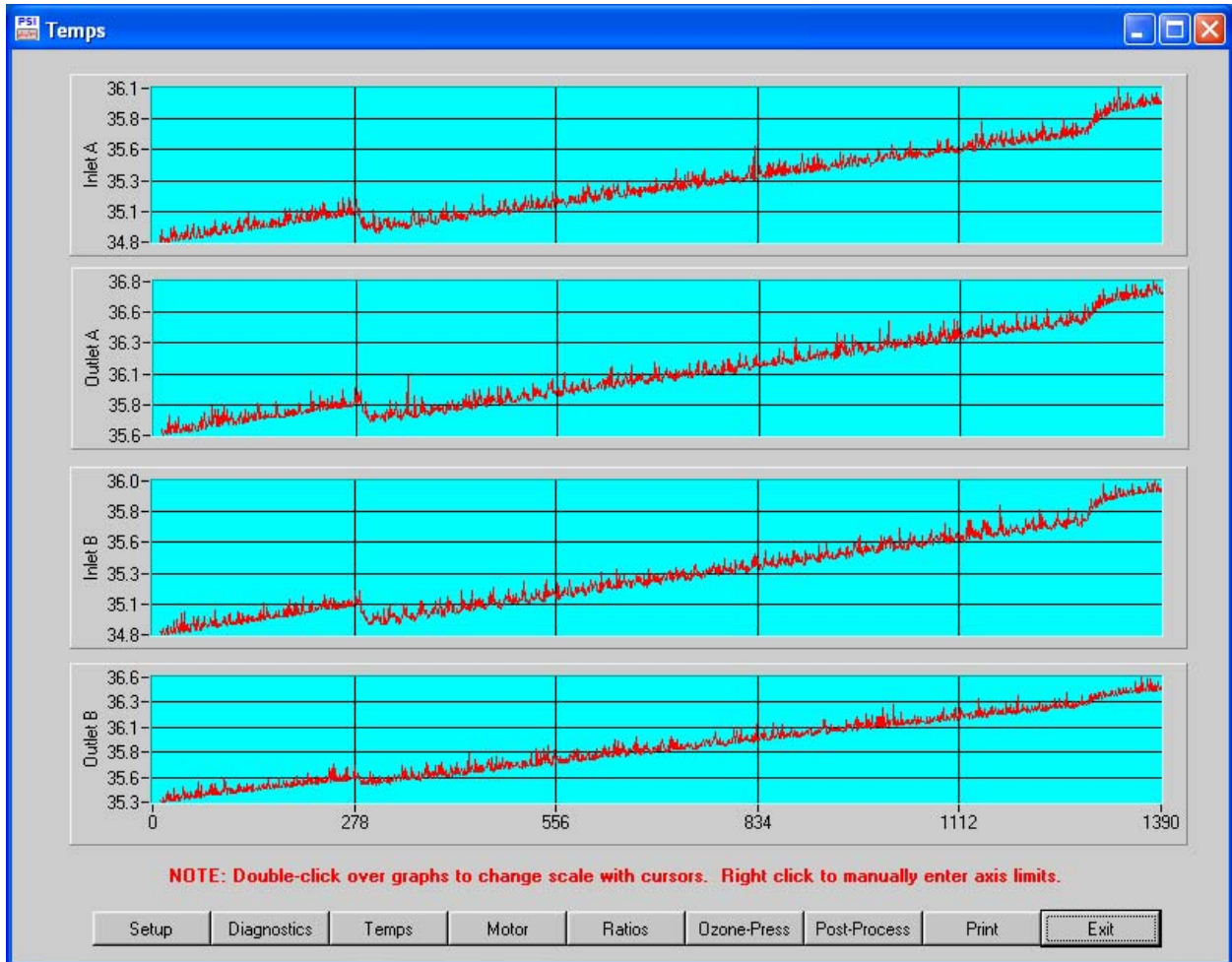
G-3. BATCH Temperature Plots: sample air inlet and outlet temperatures for Channels A and B.
