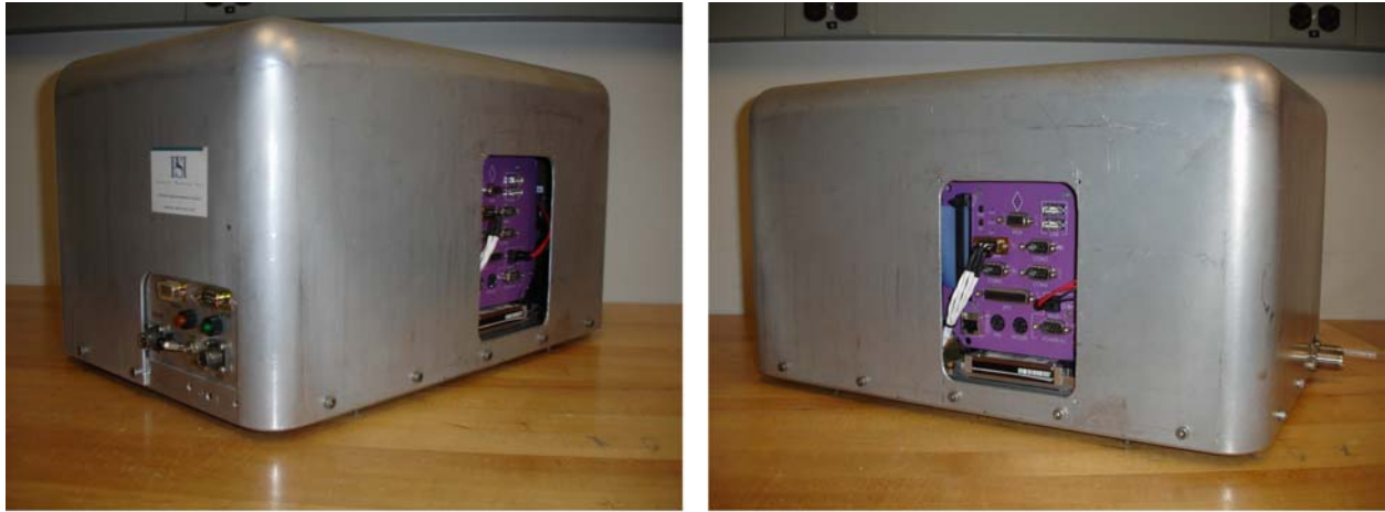
Figure 15. Instrument with housing cover installed (PC-104 access panel removed).
