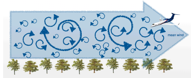
Figure 1: Wind velocity from aircraft enables measurement of eddies on scales from 10s of meters to kilometers and larger.
