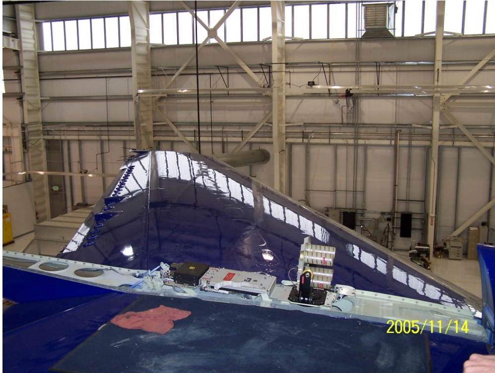
Figure 5.11: View of the GV tail deck area available for the mounting of scientific equipment
