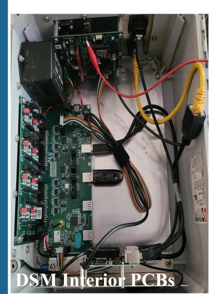
EOL has over 60 DSM (data systems) that monitor and collect data on temperature, air pressure, and wind speed. The PCB that delivers power to these sensors and the DSM CPU is unreliable at high current, due to the overheating of the switching transistor (VN5E160AS-E), which causes it to shut off. Thus, the DSM stops collecting data, until the part cools. This occurs due to a large on resistance (R<sub>on</sub>) causing high temperatures at high currents.
