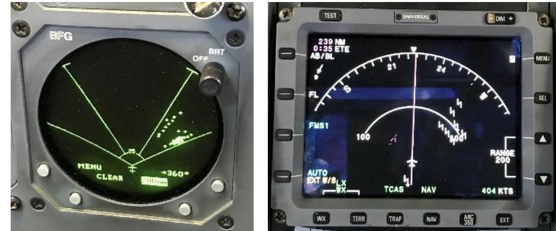
Pilot displays of Stormscope and Multi-Function Display with Radar and Lightning
