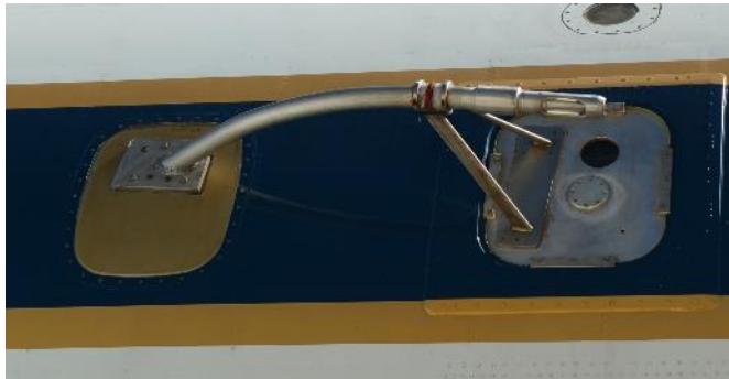
Clarke Inlet for aerosol instruments
