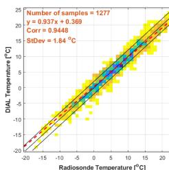
A plot of the retrieved temperature as a function of range and time is shown in the upper left-hand plot. A comparison of individual temperature profiles retrieved from the MPD and temperature profiles measured using co-located radiosondes is shown in figure to the left. A scatter plot showing the comparison of the MPD retrieved temperature with thirty nine radiosondes is shown in the upper
