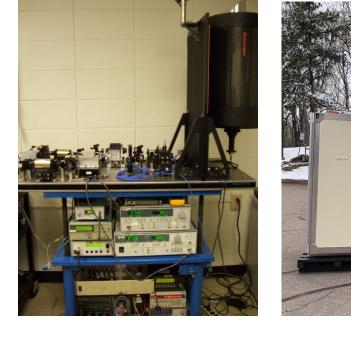
The Initial MPD instrument for humidity profiling
