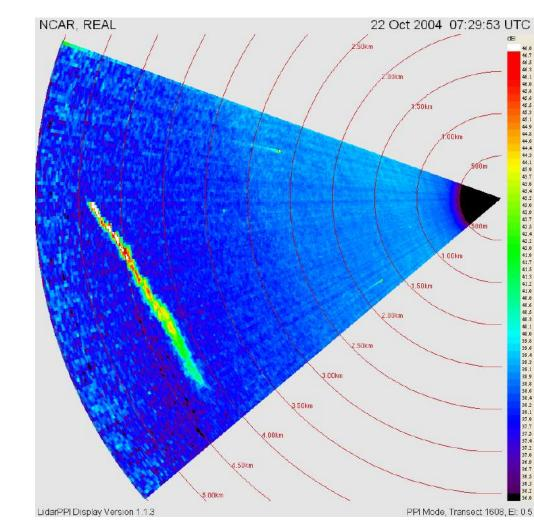
REAL is capable of detecting very small changes in particle concentration and subvisual aerosol plumes. Extensive testing was conducted for the DOD and copies of the REAL were created for national security applications.
