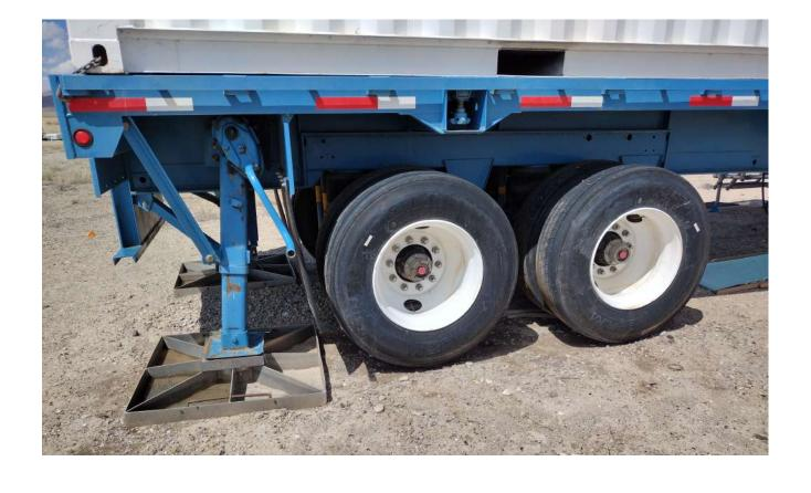
**TRAILER:** The REAL's air-ride trailer has leveling legs on each corner that allow precise leveling of the entire facility. High precision and accuracy tiltmeters monitor the pitch and roll of the trailer at all times. The system can run 24x7 and unattended in all weather conditions.
