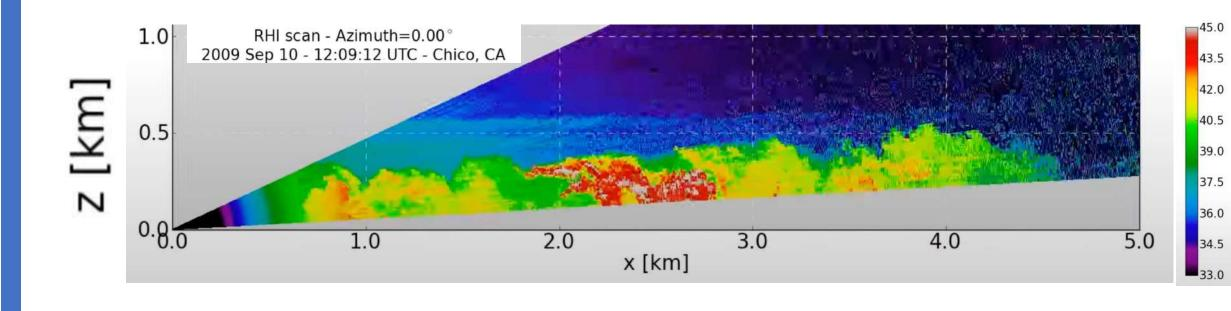
By performing rapid (15 s) RHI scans such as the one to the left, REAL excels at observing the structure and vertical evolution of convective boundary layers, especially polluted and shallow ones where the entrainment zone offers sharp contrast. A Haar wavelet-based analysis algorithm can be applied to the images to automatically and objectively delineate the top edge.
