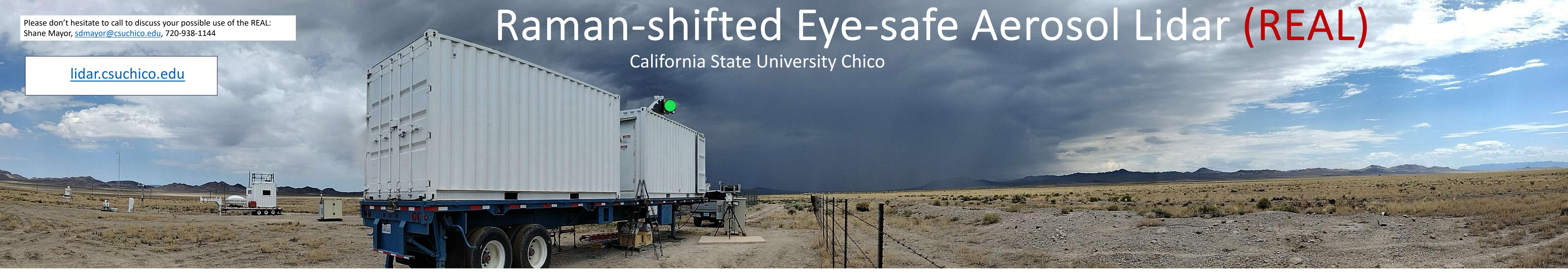
Unlike commercially available Doppler lidars and micropulse lidars, the REAL transmits very energetic laser pulses (130 mJ/pulse) at a low pulse rate (10 Hz) in order to produce images quickly. No temporal integration of the returns is required. It also transmits very short pulses (6 ns) and samples at a high rate (100M samples/s) in order to produce images with very fine range resolution (1.5 m).
