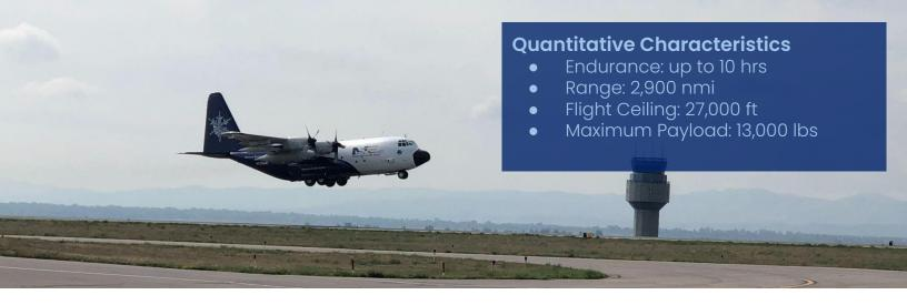
The C-130 is equipped with standard thermodynamic, wind and turbulence, microphysics, radiation, and trace gas instruments. The aircraft has a roomy fuselage with a sizable payload area, and can be equipped with a variety of versatile inlets, optical ports, and several wing pods. This allows the aircraft to carry advanced NCAR and community instrumentation, including the AVAPS Dropsonde system, the Wyoming Cloud Radar, and the Wyoming Cloud Lidar.
